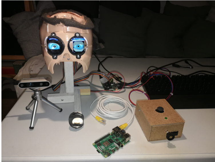
Figure 2.1: Overview of all equipment setup in this prototype. One eye lens is removed to demonstrate the LCD monitor behind it. Depth camera can be seen below, to the side of the head prototype. Raspberry Pi 3 running the eyes can be seen in the background.
