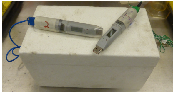
Figure 3.12 Cement slurries being locked on the top during three days temperature logging
