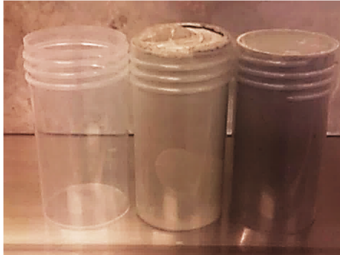
Figure 3.13 Cement mold cup, cement filled and top unpolished, cement top polished for testing
