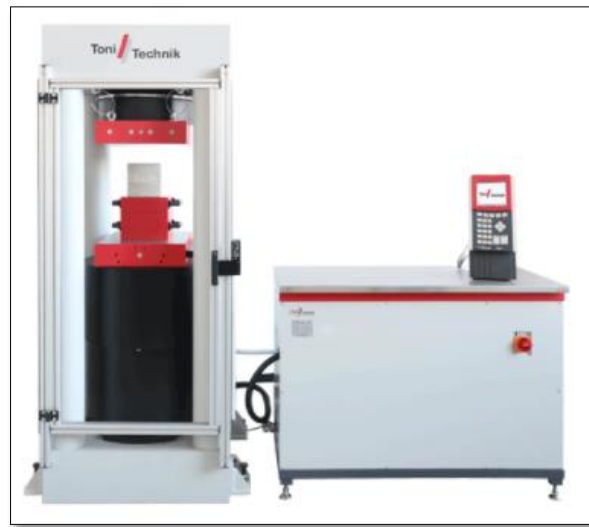
Figure 3.8 - Equipment Used to Measure UCS
