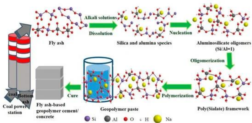
Figure 1- Mechanism and synthesis of geopolymer [10]
