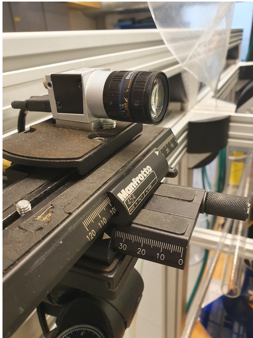
Figure B.16: Basler Ace 510, used to carry out PIV measurements
