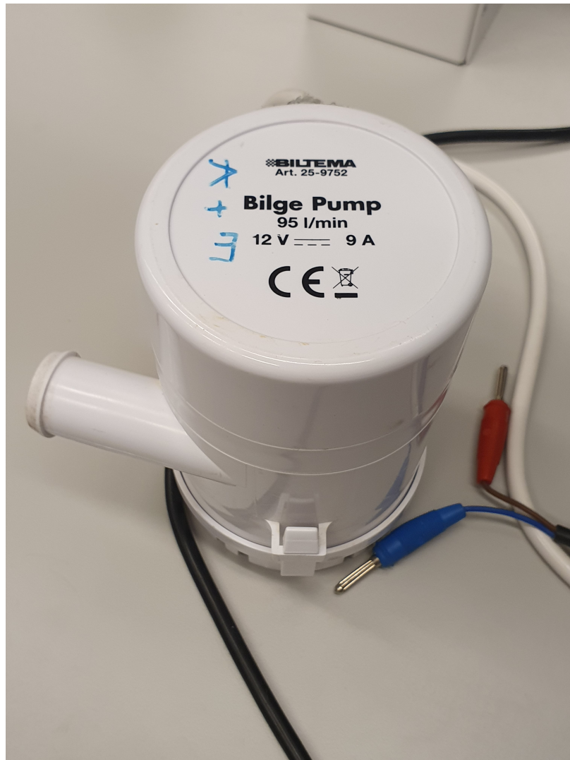
Figure B.8: Bilge pump 95 L/min, used to provide flow to the system
