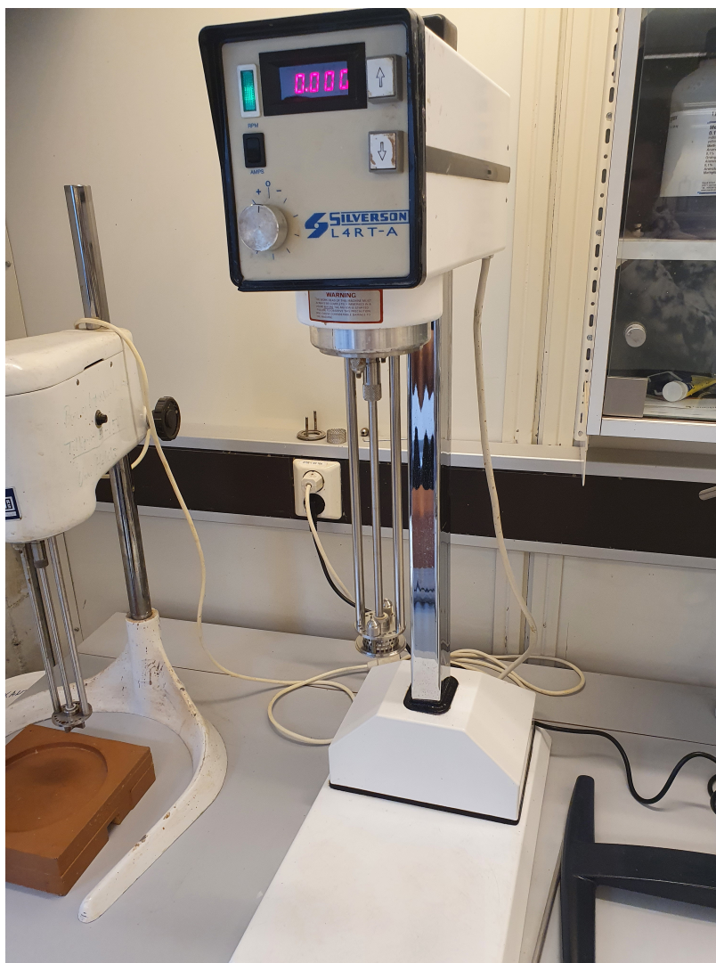
Figure B.4: Silverson L4RT-A, used to mix the fluids
