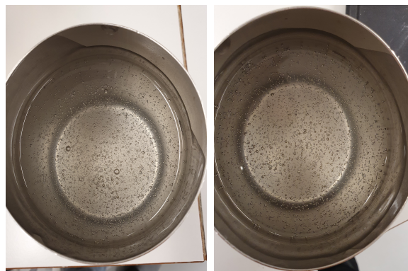
Figure A.1: Air bubble comparison. Left is original sample; right is the next day.
