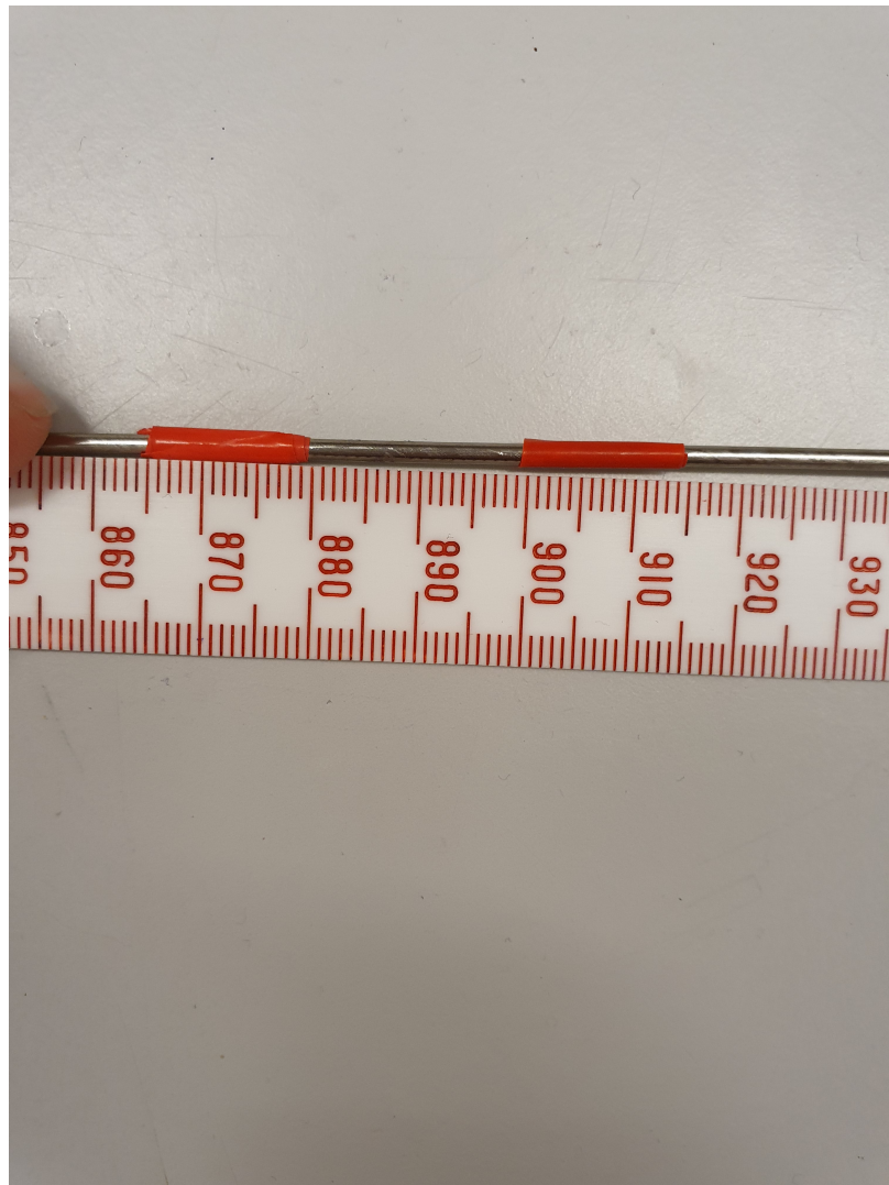
Figure B.15: Measuring calibration rod to 20 mm
