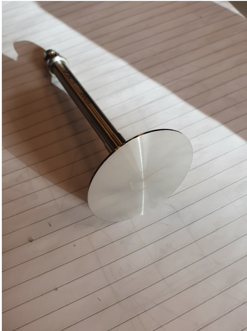
Figure B.7: CP50-1, cone-plate used in MCR 302. Diameter = 50 mm, \alpha = 1^\circ
