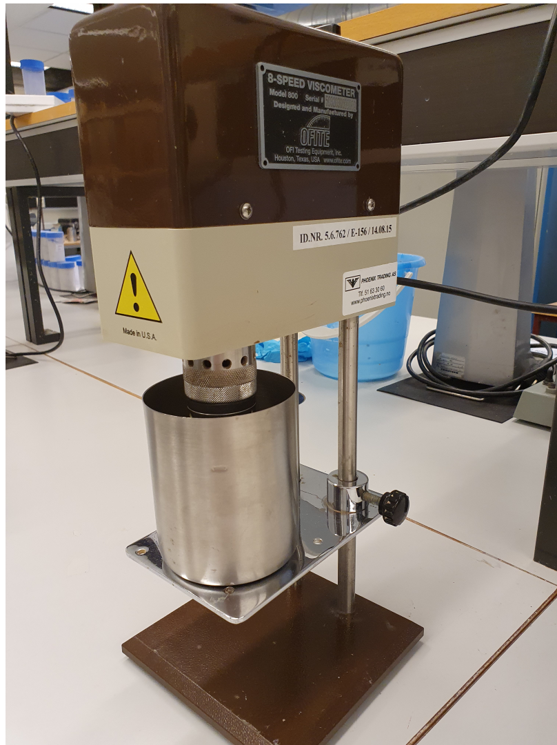
Figure B.5: 8-speed viscometer model 800, the V-G meter used to study shear stress
