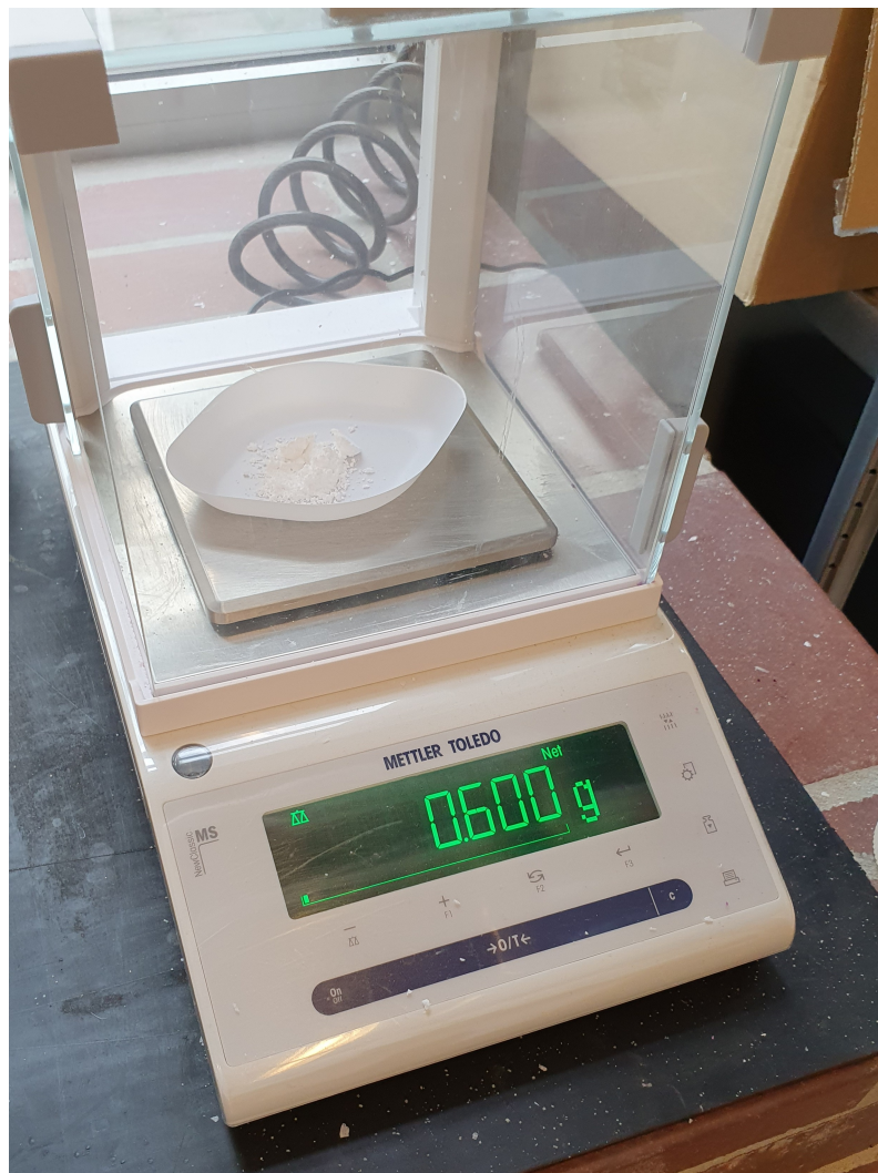
Figure B.2: Mettler Toledo NewClassic MS, used to accurately measure Carbopol
