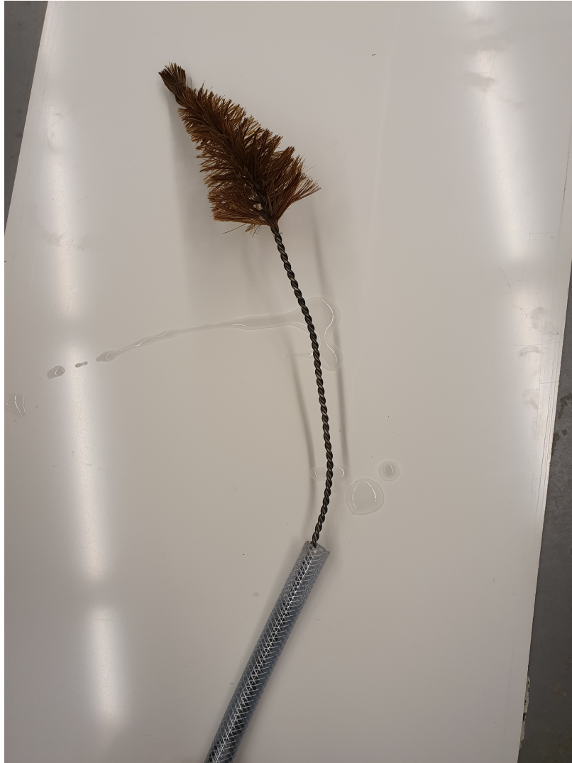
Figure B.13: conic pipe-brush, used in between PIV measurements to remove air bubbles or seeding material inside pipe
