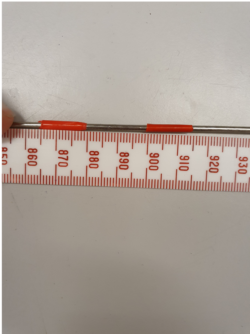
Figure B.15: Measuring calibration rod to 20 mm
