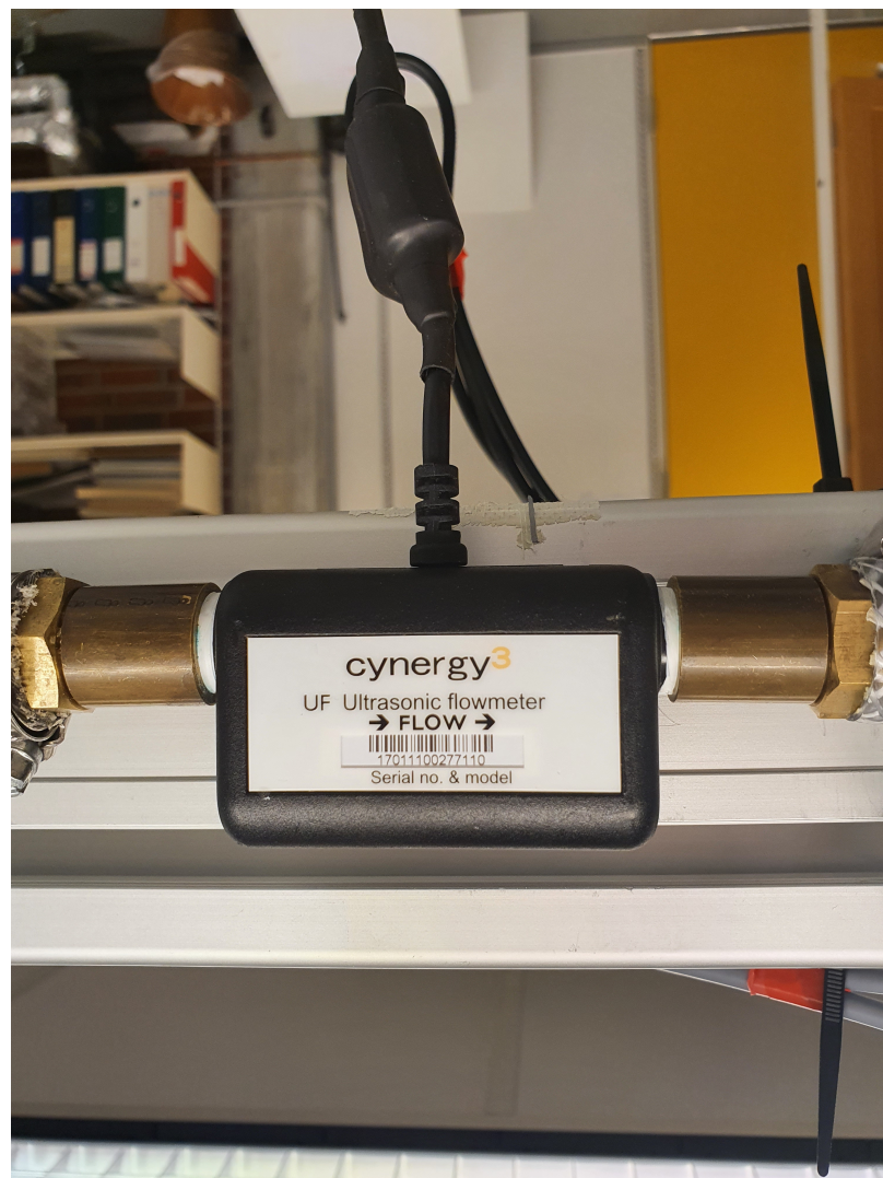
Figure B.11: Cynergy 3 Ultrasonic Flowmeter, measured the flowrate for the system
