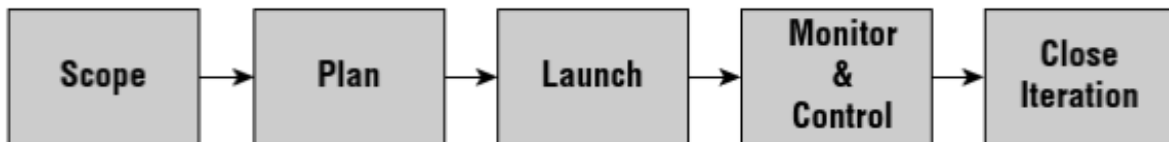
Figure 2.1: The Linear Project Management Life Cycle model (Source: (Wysocki, 2014, p. 43))
