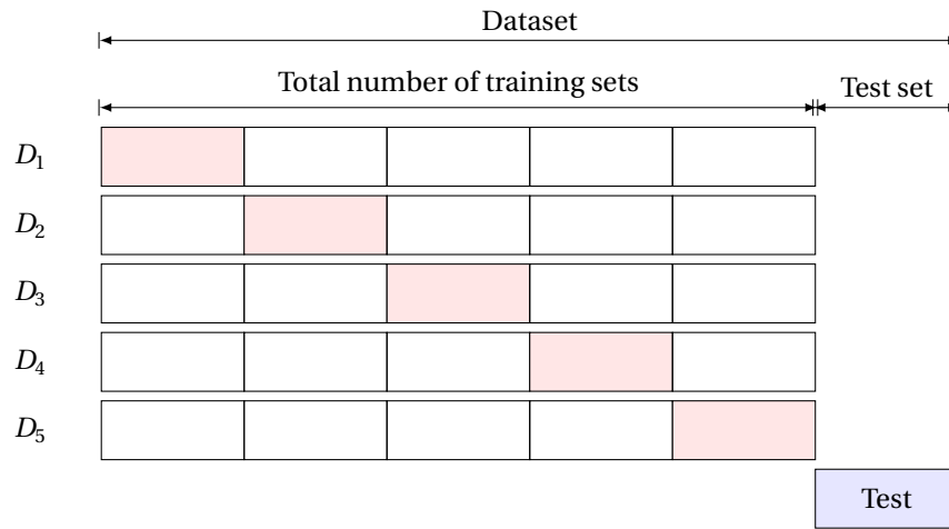
Figure 2.8: Cross validation. The red rectangles represent the dataset that is used for testing the model (temporary test set) when trained on all the other four white ones on that line, based on the results for these the hyperparameters for the model is set. Then the model is trained on all the training set. The test set is used when all parameters are decided after the cross validation
