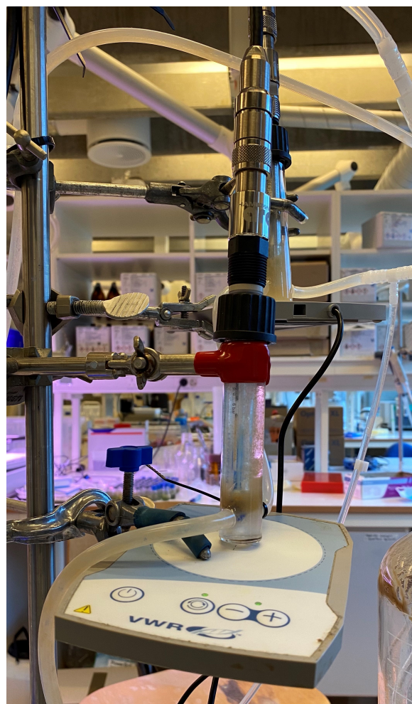
(b) pH sensor placed within a flow cell.
