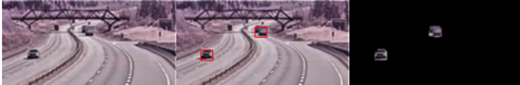
Figure 13: Capturing an image, detecting the objects in motion, and extracting them.
