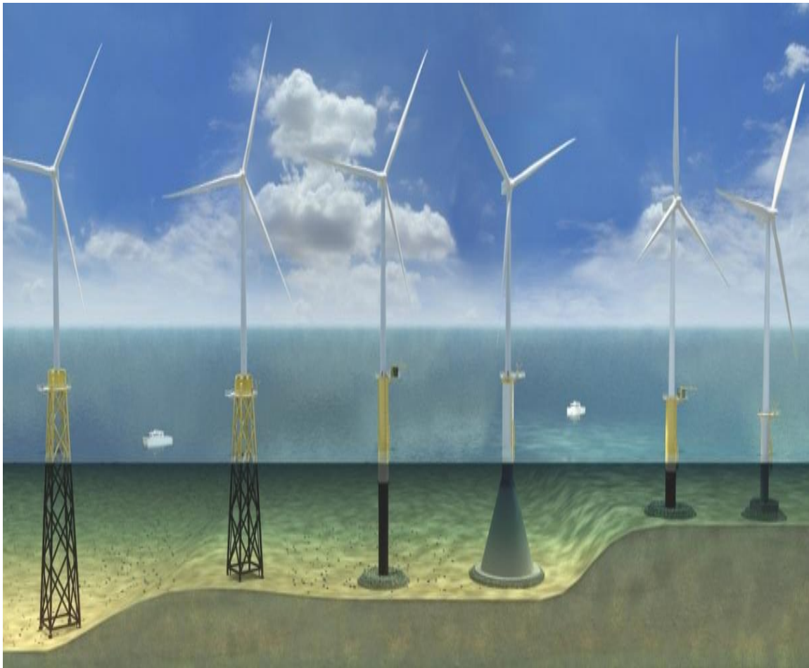
Fig.2.3: Bottom fixed foundations for wind turbines (google.com. 2021)
