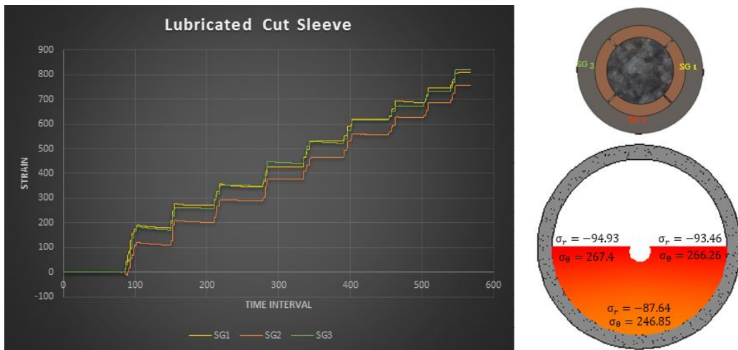
Figure 3.14: Lubricated cut sleeve with SGs at 0°, 270° and 180°
