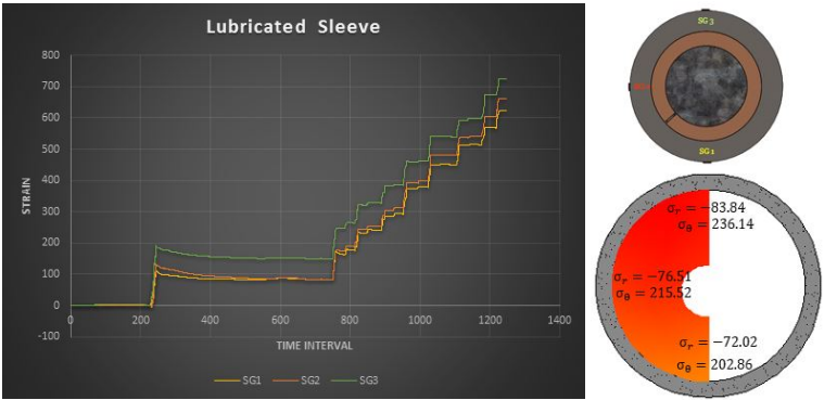
Figure A.6: Lubricated sleeve with sleeve complete notch at 225° and SGs at 270°, 180° and 90°
