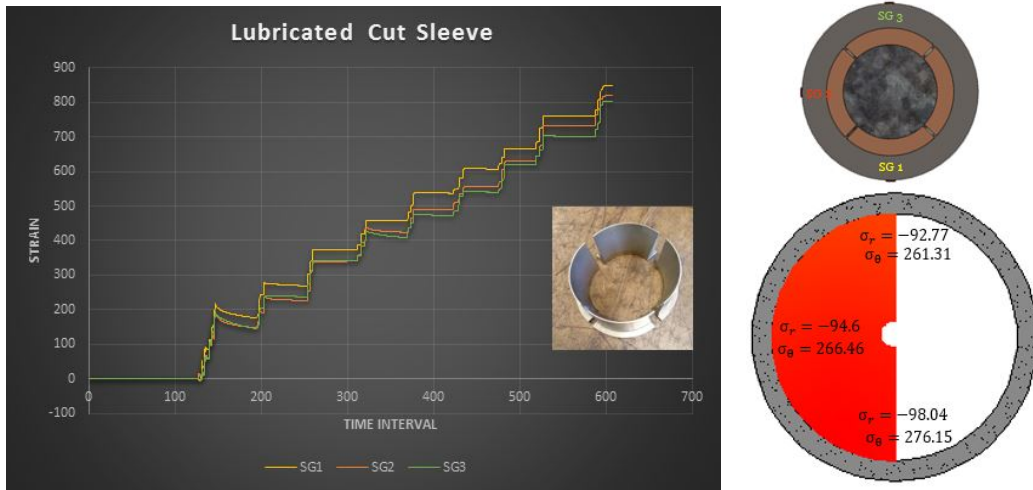
Figure 3.13: Lubricated cut sleeve with SGs at 270°, 180° and 90°
