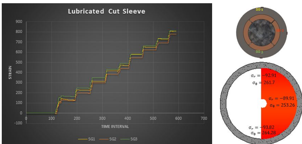
Figure 3.15: Lubricated cut sleeve with SGs at 90°, 0° and 270°
