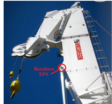
Figure 6.1: Bondura® EPS application in crane [1]
