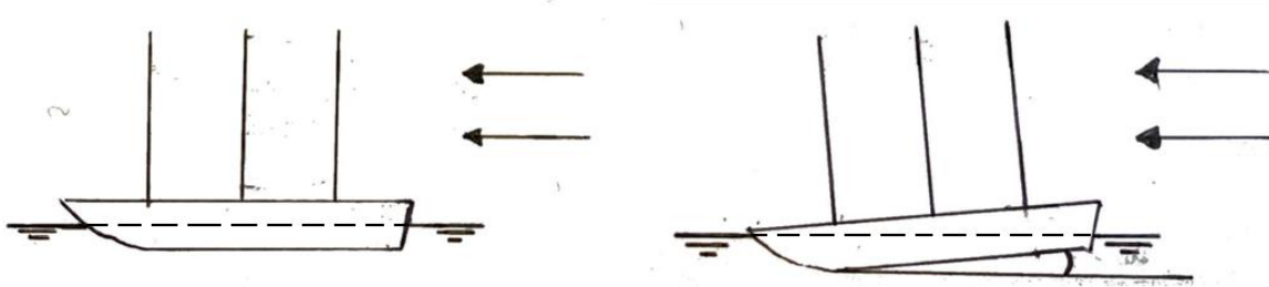
Figure 4.2 - Rotation towards bow due to wind forces from aft position. Not an accurate representation.
