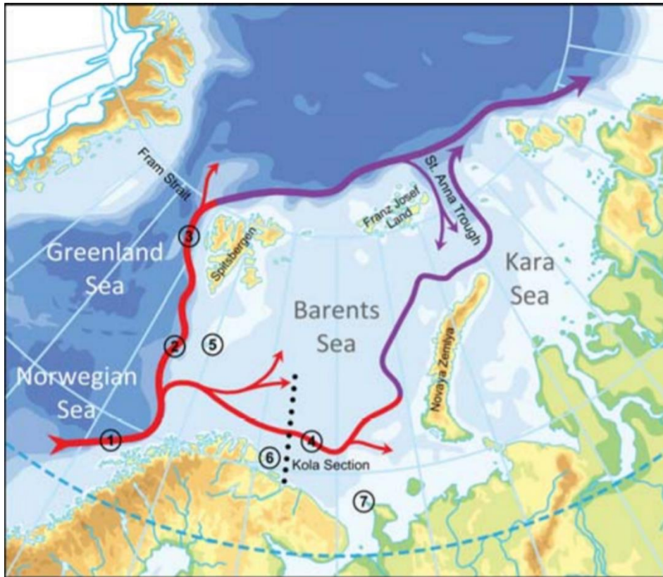
Figure 2.6 The main directions of currents in the Barents Sea 1. Eastern branch The North Cape current. 2. Spitsbergen current; 3. West Spitsbergen current; 4. Murman current [8]
