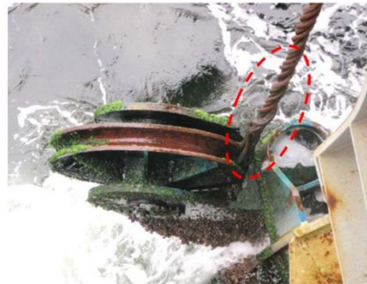
Figure 5.12. Damage wire rope in fairlead [32]
