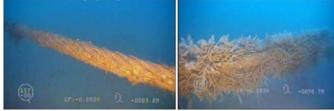
Figure 5.2. Underwater inspection of wire rope [2]
