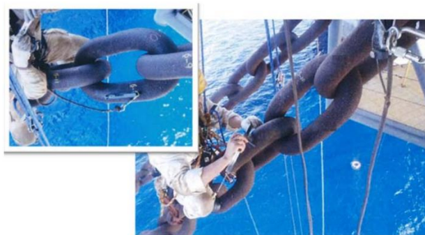
Figure 5.4. Diameter measurement of chain with caliper [25]
