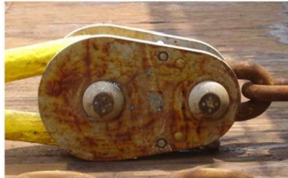
Figure 2.11. H-shackle connecting polyester rope and chain [16]
