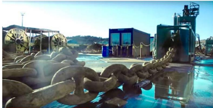
Figure 5.1: Dockside inspection method for MODU chain [6]
