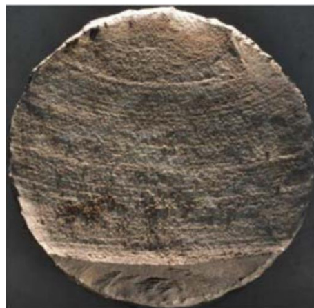
Figure 4.1. Broken surface showing beach marks [2]
