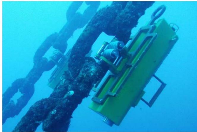
Figure 5.9. Inclinometer installed on top of chain [2]
