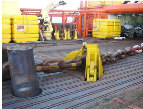
Figure 3.16. chain gets pulled through the towing pins (left) on the deck and secured by the shark jaw (middle) [2]
