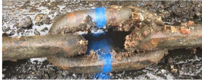
Figure 5.6. Ground chain and touch down chain with lose of material in one side [25]
