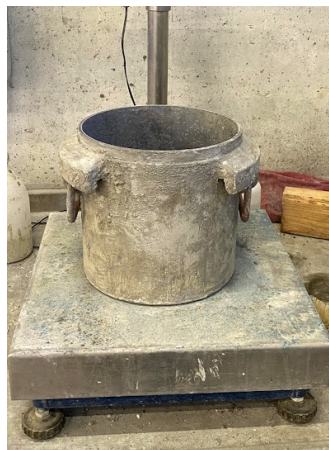
Figure 3.16: Density of fresh concrete
