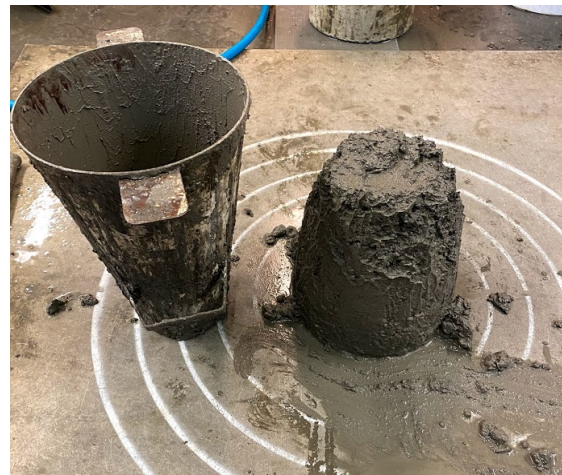
Figure 3.15: Slump of concrete
