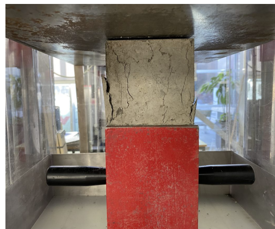
Figure 3.21: Fracture due to compressive strength testing
