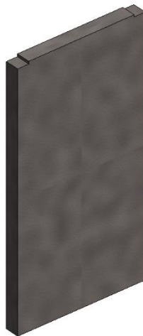
Figure 35 Reinforced concrete wall
