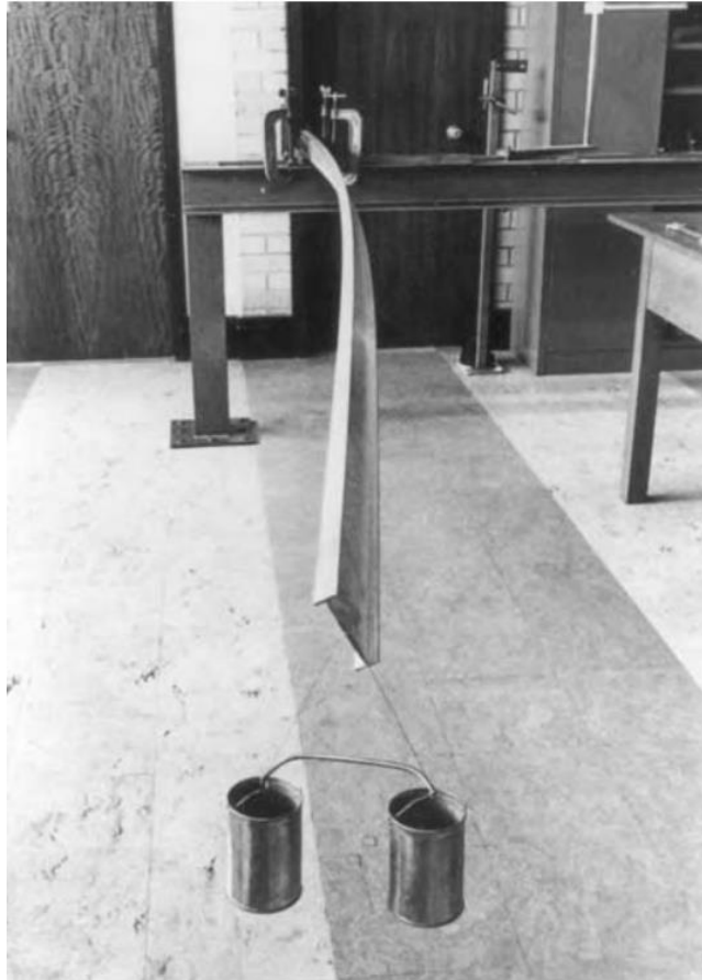
Figure 2.1-2: Lateral Buckling of a cantilever [9]
