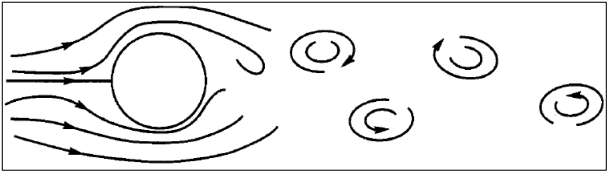
Fig. 3.6. Vortex shedding after the cylindrical body
