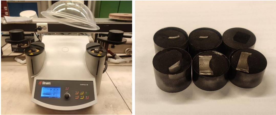
Figure 45: (a) Struers Citopress-30 (b) Hot mounted sample
