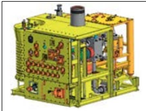
Figure 3–4 Three-dimensional model of the X-mas tree [25]
