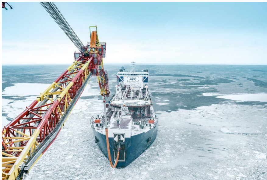
Figure 5–11 Offloading of oil using DOOU [46]
