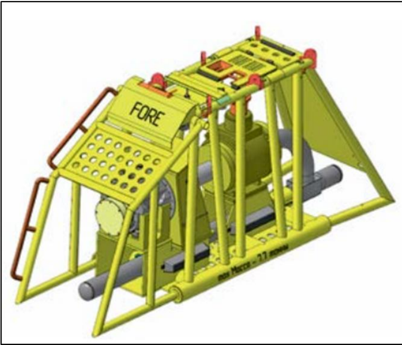
Figure 3–3 Three-dimensional model of a DN200 inline tee [22]
