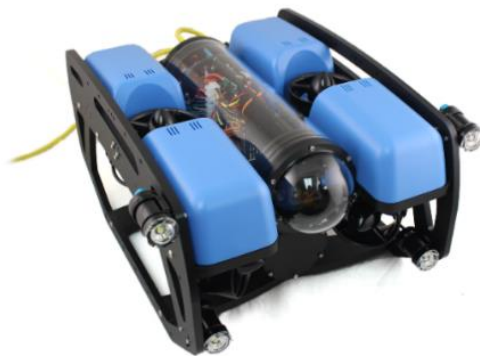
Figure 1-3 BlueROV2 base version (BlueRobotics 2021)
