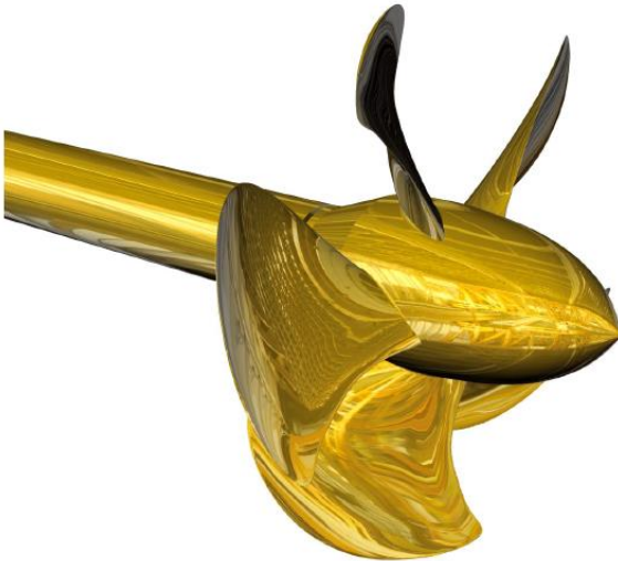
FIGURE 80 PROPELLER VP1304 AS TURBINE WITH FRONT MOUNTED STEM [41]
