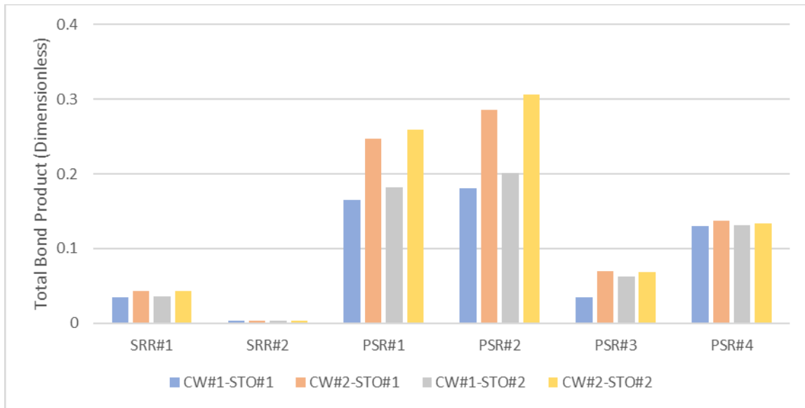
Figure 4. 14: Prediction of the oil-adhesion tendencies of reservoir rocks and mineral mixtures using the total bond product during CWI.
