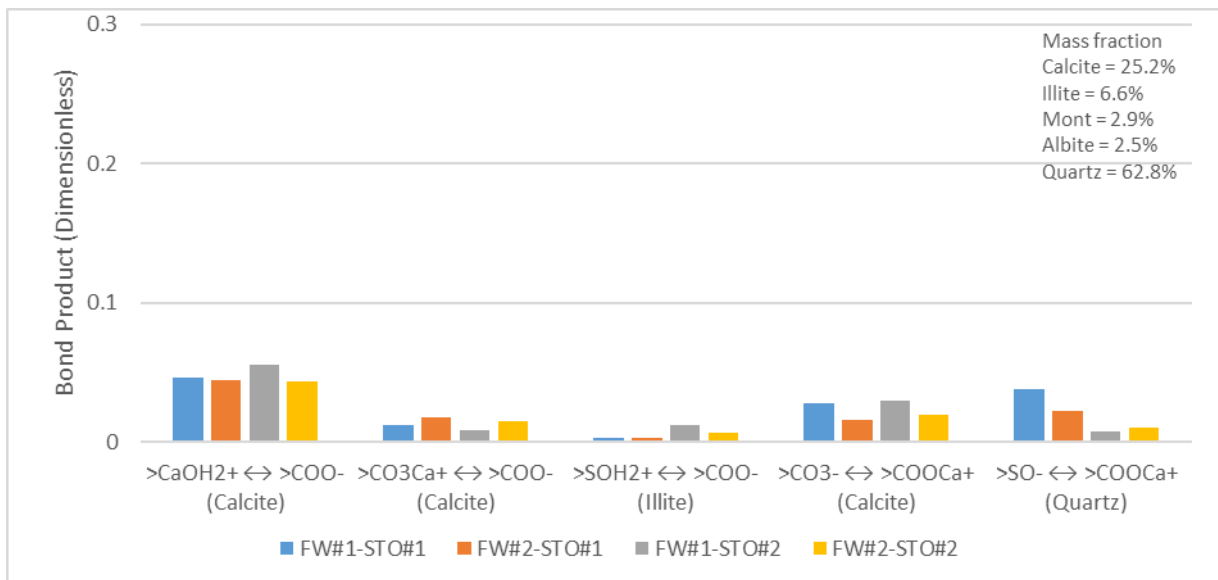
Figure 4. 23: Prediction of the oil-adhesion tendency of PSR#3 using the bond product during FWI.
