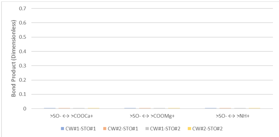
Figure 4. 6: Prediction of the oil-adhesion tendency of albite using the bond product during CWI.
