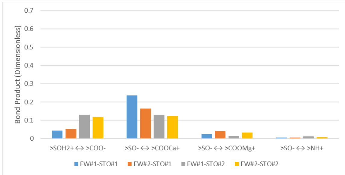
Figure 4. 9: Prediction of the oil-adhesion tendency of montmorillonite using the bond product during FWI.
