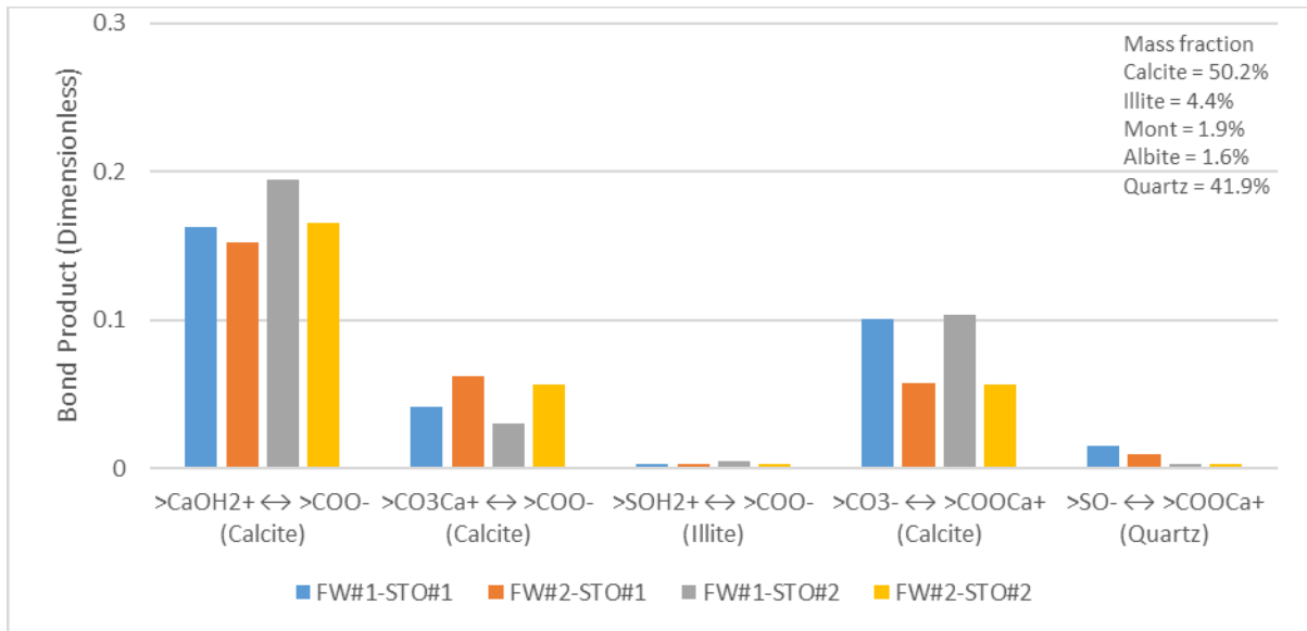
Figure 4. 24: Prediction of the oil-adhesion tendency of PSR#4 using the bond product during FWI.
