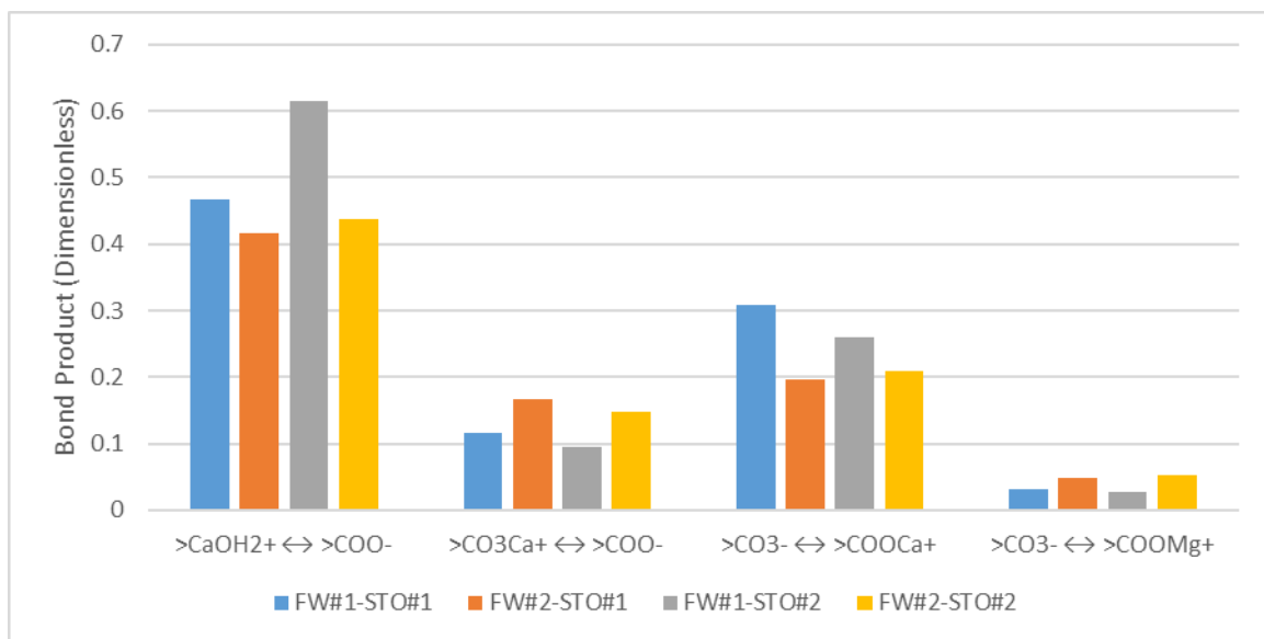
Figure 4. 11: Prediction of the oil-adhesion tendency of calcite using the bond product during FWI.
