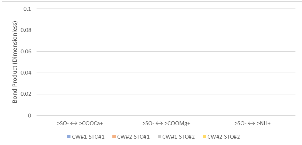
Figure 4. 4: Prediction of the oil-adhesion tendency of quartz using the bond product during CWI.
