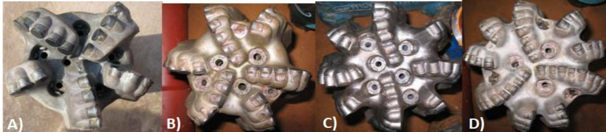
Figure 2.4: PDC bit design for varying formation hardness (from soft (A) to hard (D)) [35]
