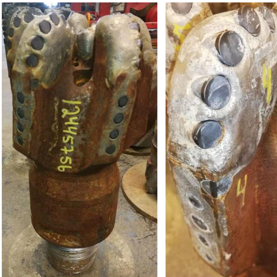
Figure 2.30 - PDC bits: One-step gauge pad bit
