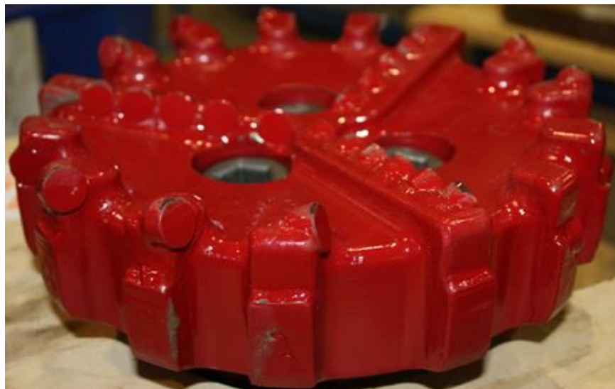
Figure 2.25 - PDC bits: Pancake drill bit
