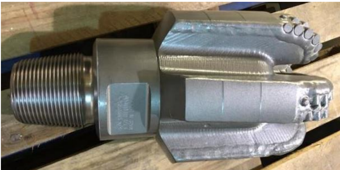
Figure 2.28 - PDC bits: Stepped gauge pad bit
