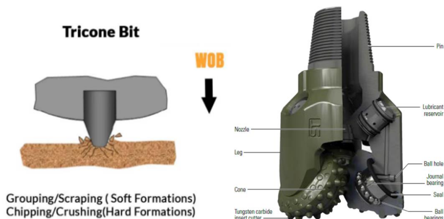
Figure 2.15 - Roller cone: Tricone Bit
