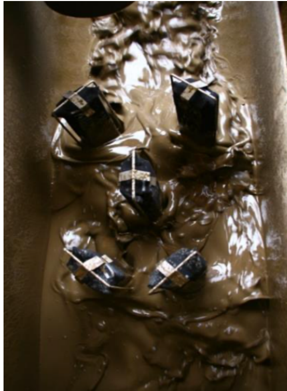
Figure 21 – Ditch magnet system (Strømø 2016)
