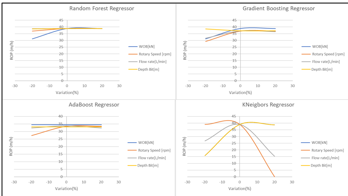
Figure 30: Sensitivity analysis case 2 for ROP models.
