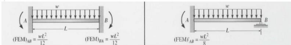
Figure B-3: Simplified bending moments for end and mid spans, screenshot from "Structural Analysis", R.C. Hibbeler
