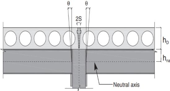
Figure 2-23 Element rotation at support [23]
