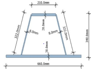
Figure 5-3 Steel beam D32-400
