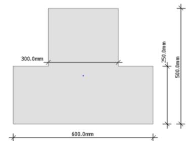
Figure 5-6 Concrete inverted T-beam (600x500)
