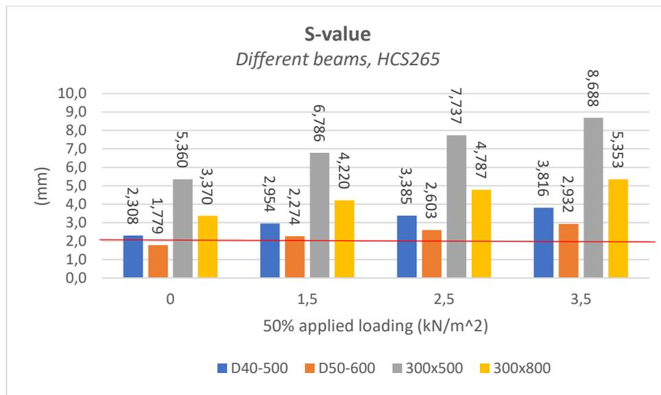
Figure 5-11 S-value for different beams with a HCS 265
