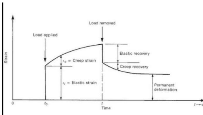
*Figure 3-1 Creep in concrete*
