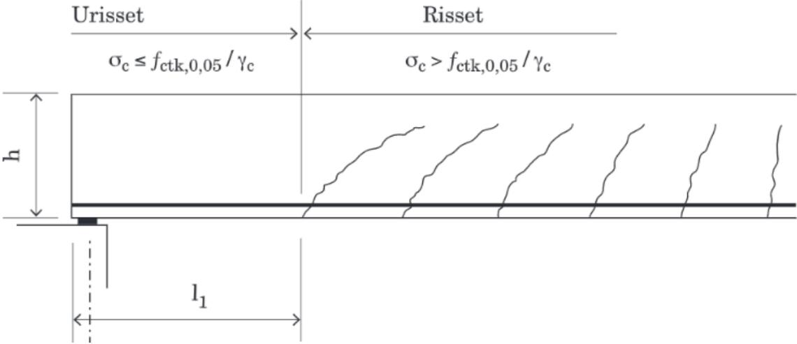
Figure 2-16 Area uncracked by bending [2]
