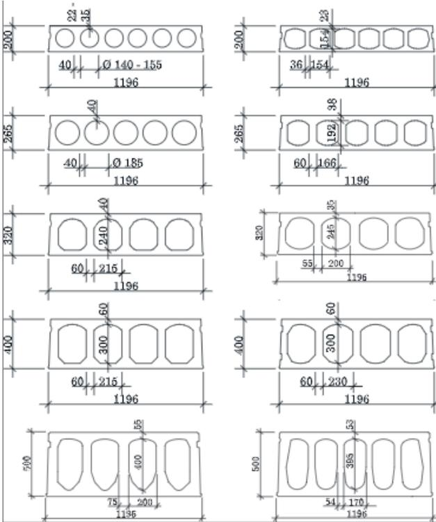
Figure 2-1 Different cross-sections of hollow core slabs [2]
