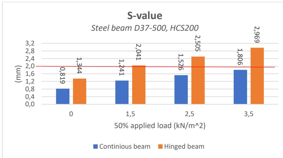
Figure 5-9 S-value for steel beam D37-500
