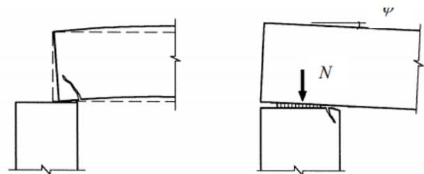
Figure 2-6 Movement in the precast elements damaging the connection [6]
