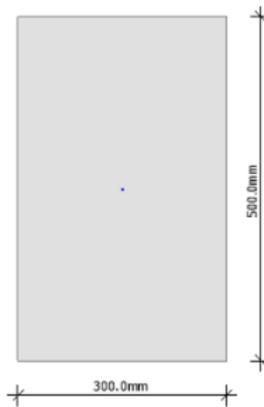
Figure 9-14 Concrete beam 300x500
