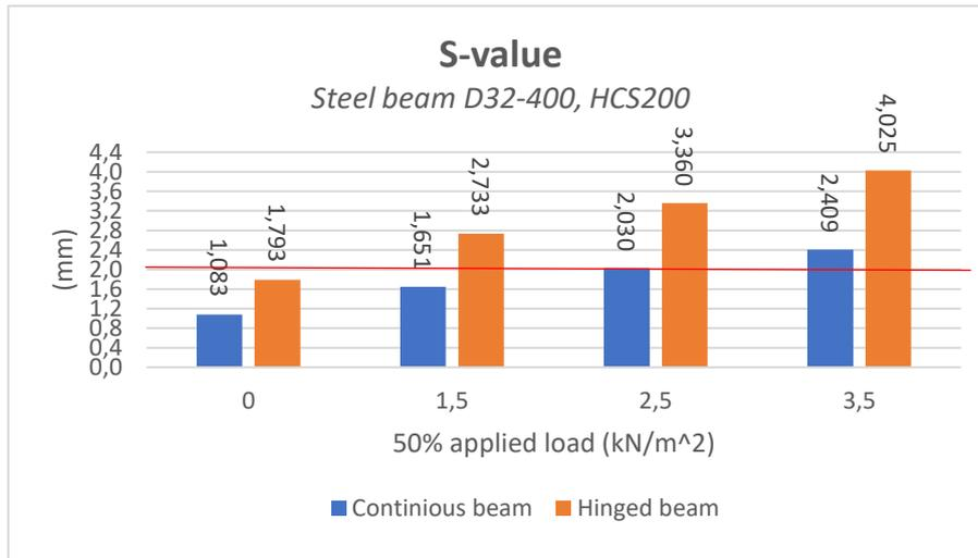
Figure 5-8 S-value for steel beam D32-400
