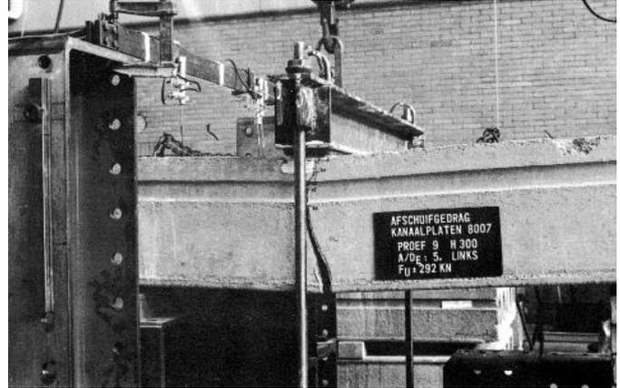
Figure 2-12 Anchorage failure [9]
