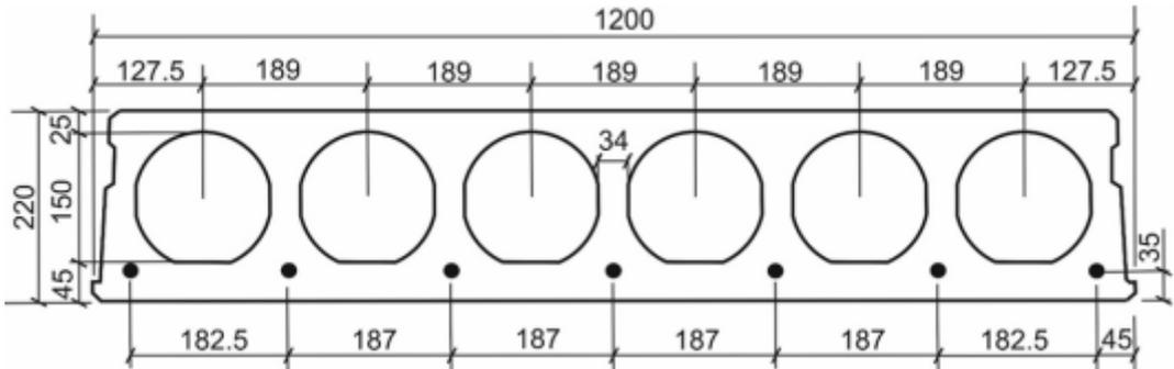
Figure 2-2 Reinforcement strands in hollow core slab [4]
