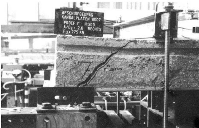
Figure 2-15 Shear tension failure [9]
