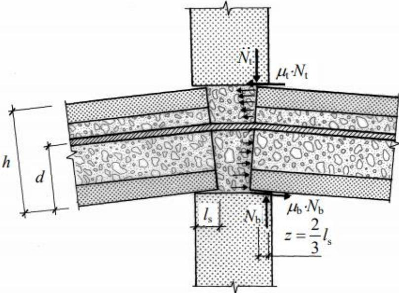
Figure 2-7 Example of cause of unintended restrain in connection [6]
