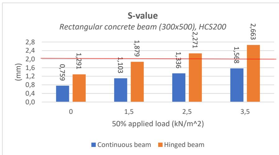
Figure 5-10 S-value for rectangular concrete beam (300x500)
