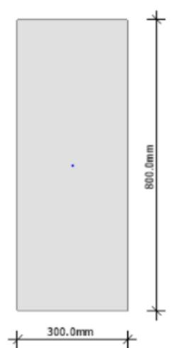
Figure 9-12 Concrete beam 300x800
