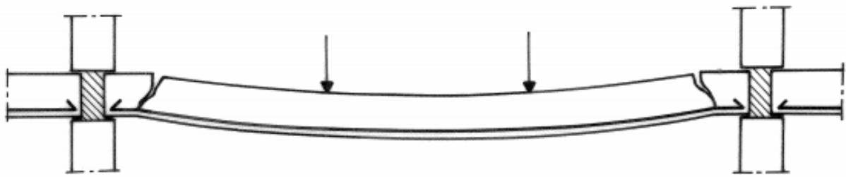
*Figure 2-8 Restraining of the connection, leading to a negative moment at the support [6]*
