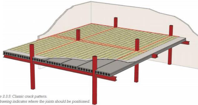
Figure 2-24 Cracking pattern in hollow core slab. The lines indicate where cracks most likely happen [23].
