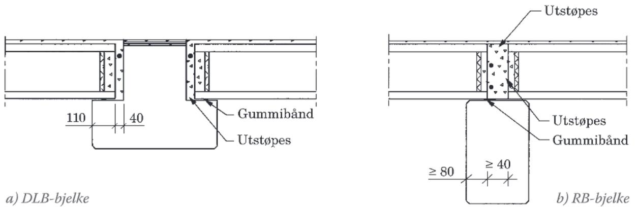
Figure 2-4 Support of hollow core slab on beam [2]
