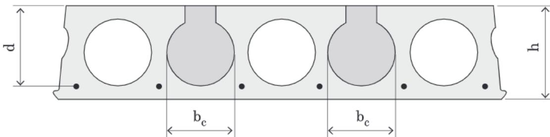
Figure 2-18 Cross-section of a hollow core slab [2].
