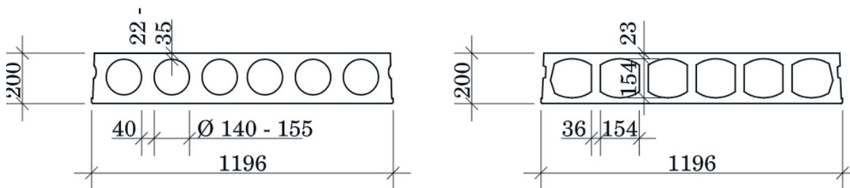
*Figure 2-20 Different shape of cross-section in hollow core slab [2]*
