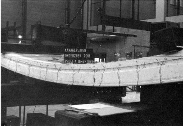
Figure 2-13 Pure flexural failure [9]
