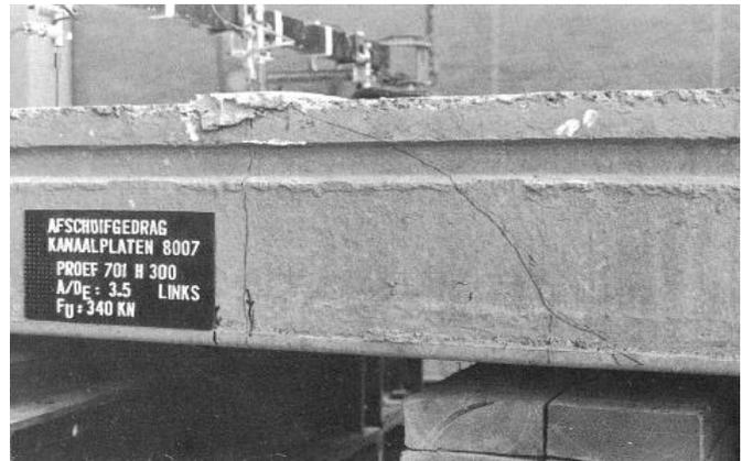
Figure 2-14 Shear compression failure [9]
