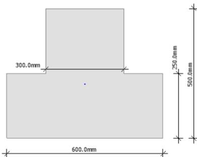
Figure 9-13 Concrete inverted T-beam (600x500)
