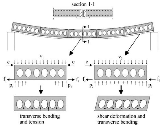
Figure 2-17 Stresses in hollow core slab on flexible support [10].
