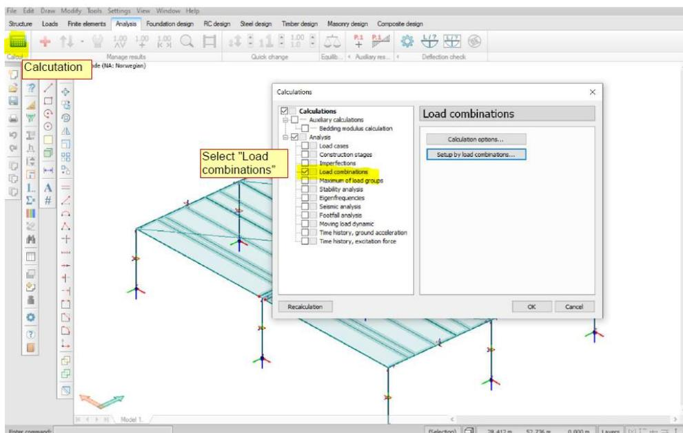
Under the analysis option, the model is calculated to see if the statics are correct. Here the deflections are calculated, and these can be used to compare to hand calculation, to see if the model can be trusted.
