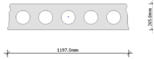
Figure 9-15 Hollow core slab 265
