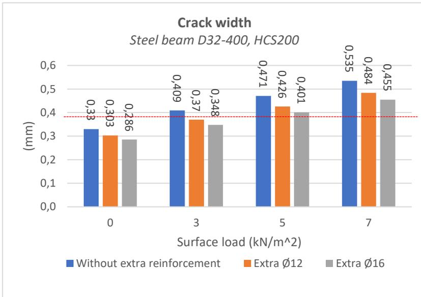
Figure 5-4 Crack width for steel beam D32-400, HCS200
