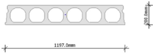
Figure 9-16 Hollow core slab 200
