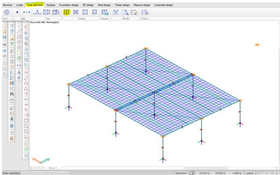
Figure 9-7 Meshing of the model
