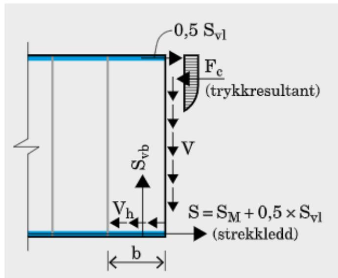
Figure 2-9 Shear forces in a slab [3]
