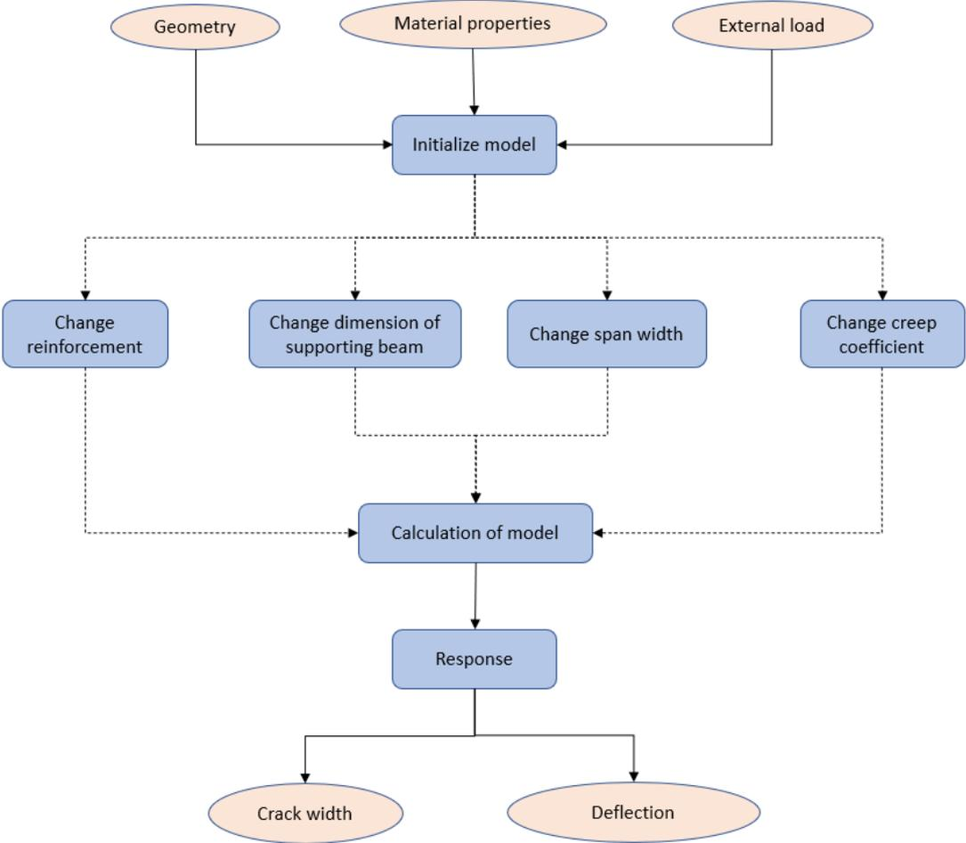
Figure 4-1 Flow chart of modelling process in FEM-design
