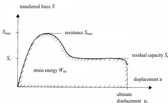
Figure 2-5 Mechanical behavior of a structural connection can be characterized by a load-displacement relationship for the primary action [6]
