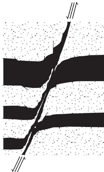
Figure 3.9: Example of Shale smear. Black layers represent the shale beds. Shale smear coming from multiple source beds into a normal fault, resulting in a more continuous shale smear. Yielding et al. (1997), modified after Weber et al., (1978).
