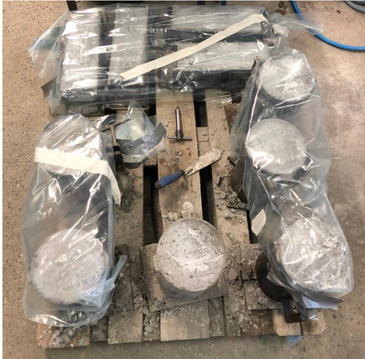
Figure 5-20 Concrete cubes and cylinders covered in plastic - The first 24 hours of curing procedure
