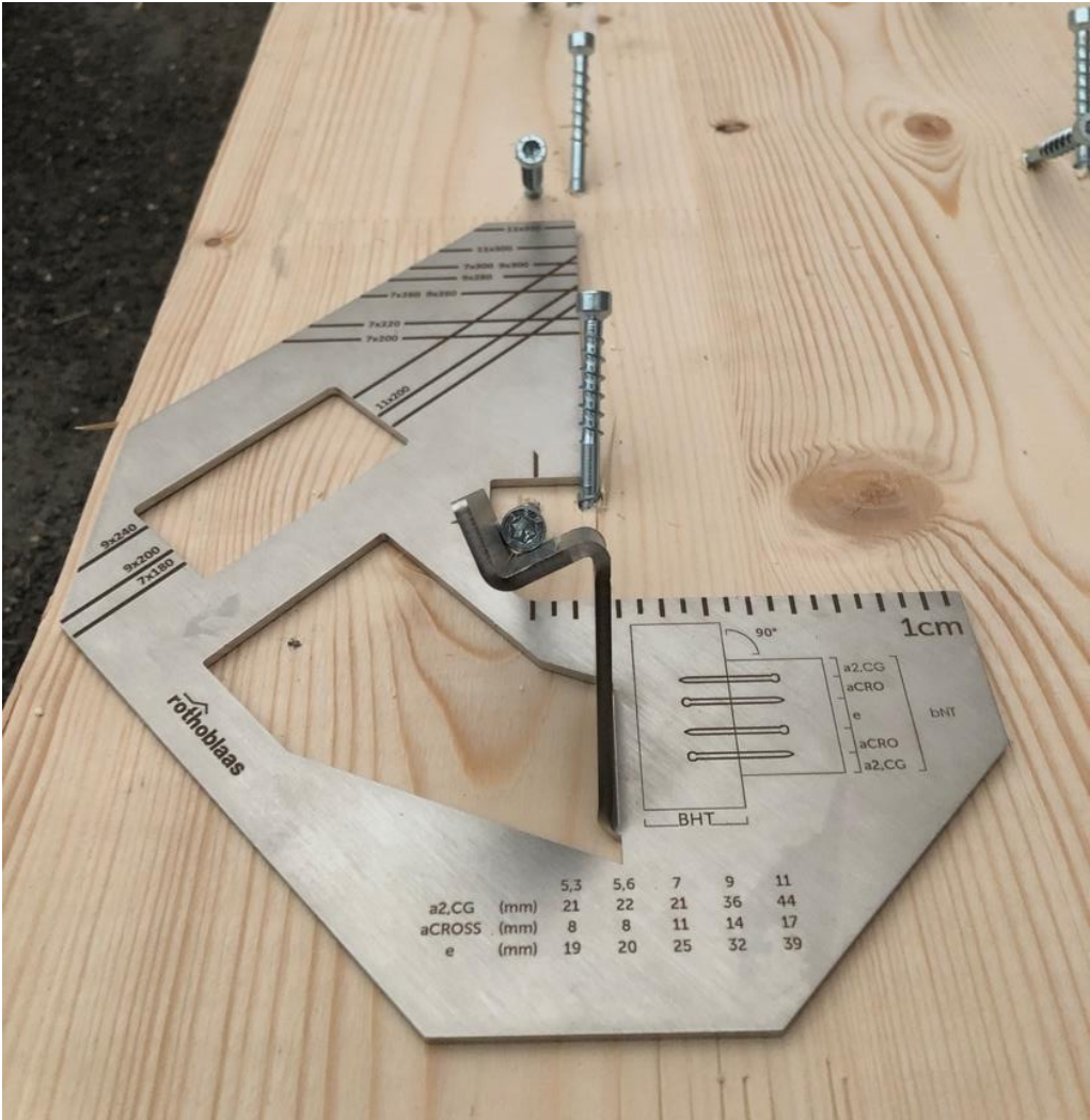
Figure 5-3 The jig used to get a 45° angle on the screws
