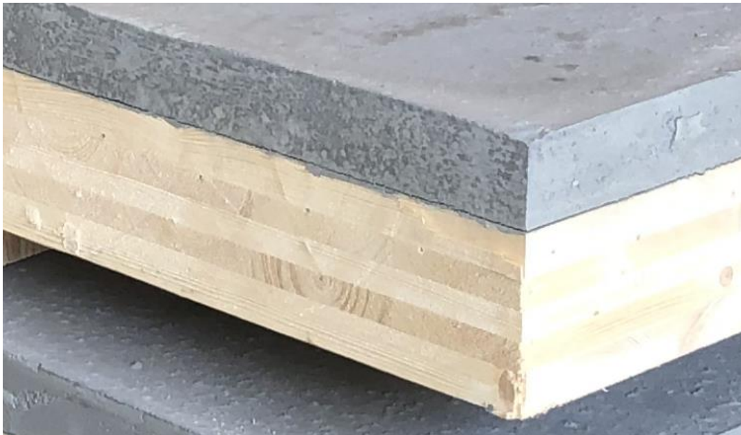
Figure 8-12 Minor gap between the concrete and timber elements before testing
