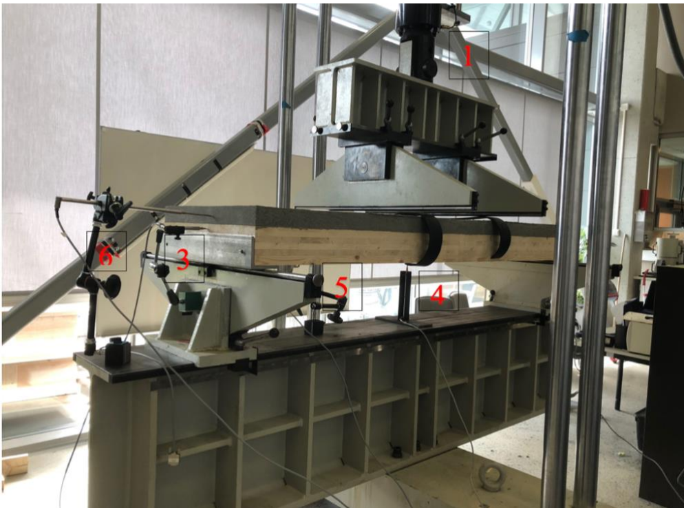
Figure 6-7 The setup for the test, LVDT's: 3, 4, 5 and 6 and load cell: 1
