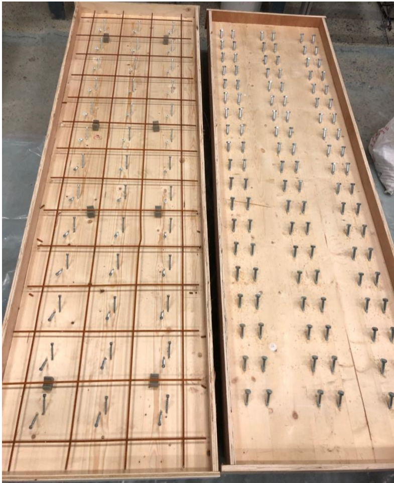
Figure 5-14 Slabs with different shear fastener and formwork surrounding the slab
