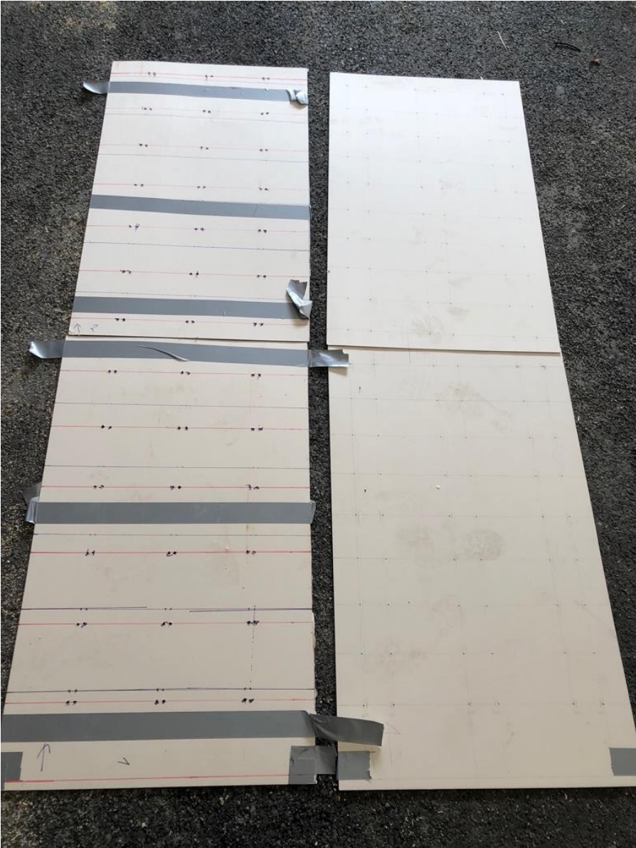
Figure 5-2 Picture of cardboard template, to the Left CTC screw template and to the Right KOP screw template
