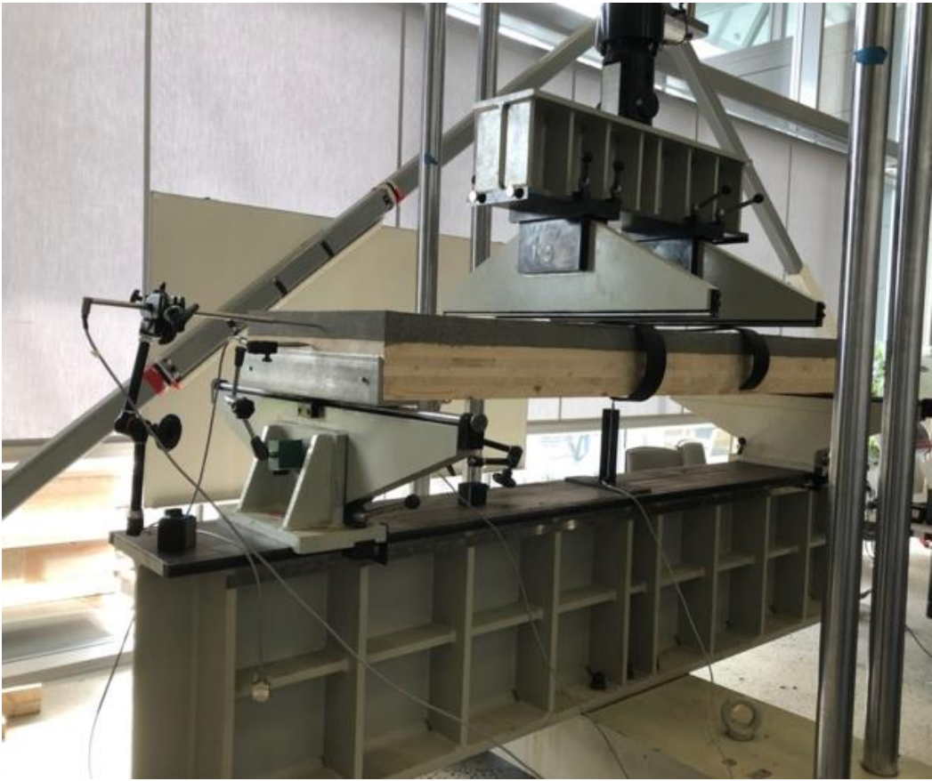
Figure 6-12 The CLT-Concrete composite slab ready for testing
