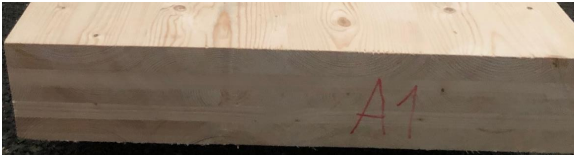
Figure 5-1 Cross section of 5-layered CLT used in laboratory testing
