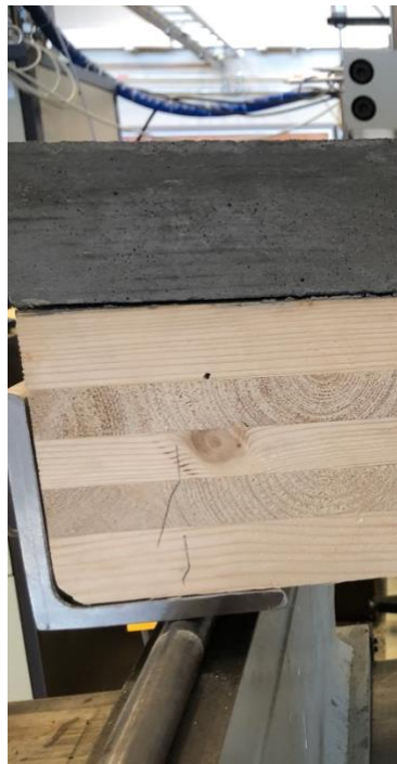
Figure 6-6 “L” shaped steel profile placed on the support, grey line marking the placement for support
