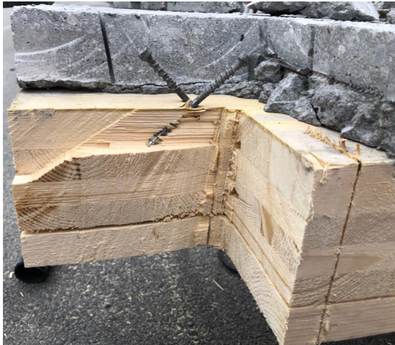
Figure 8-7 CTC screws after four-point bending test
