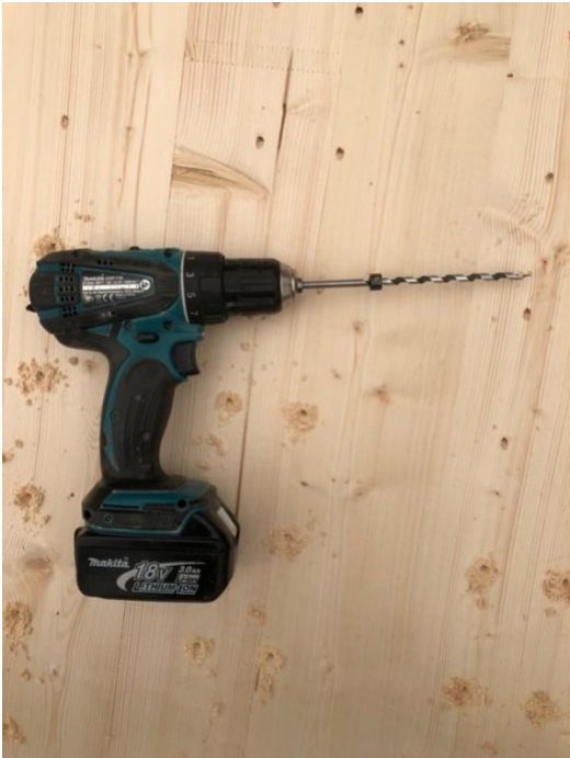
Figure 5-8 Drill with wood drill bit and with a mounted stop collar
