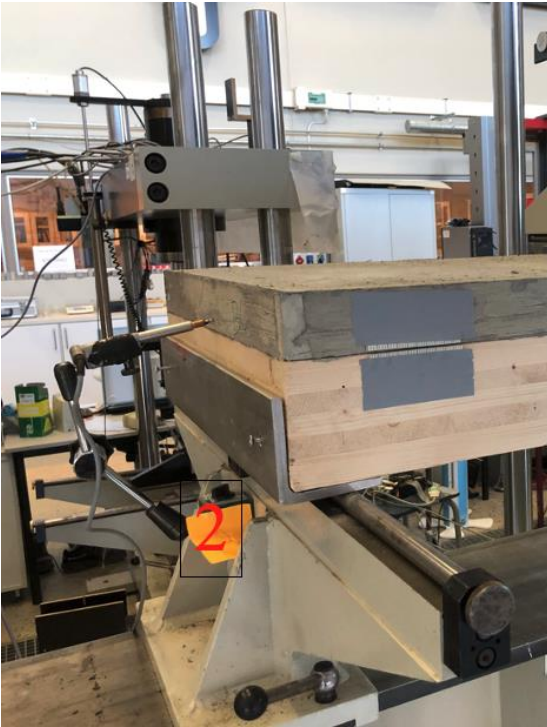
Figure 6-8 The setup for the test, LVDT 2
