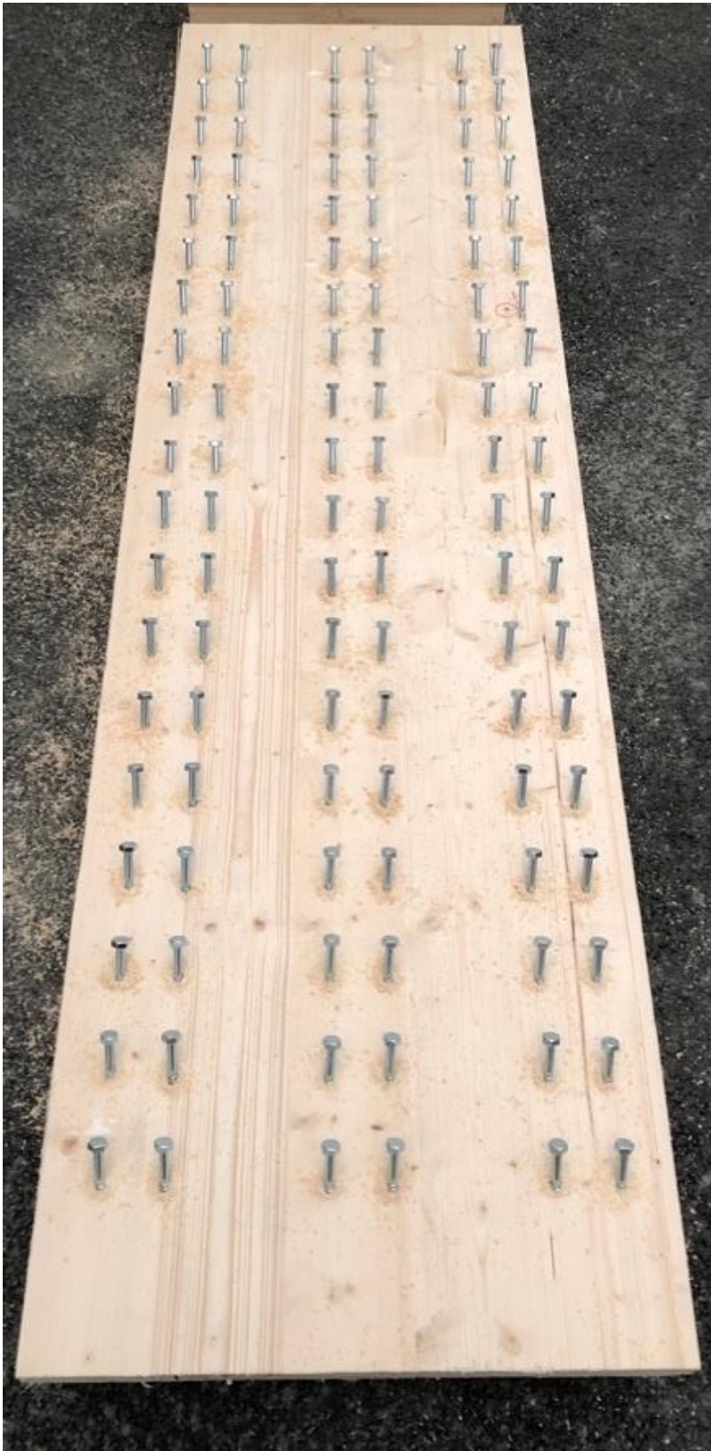
Figure 5-11 A slab with KOP screws parallel oriented with a 45° angle
