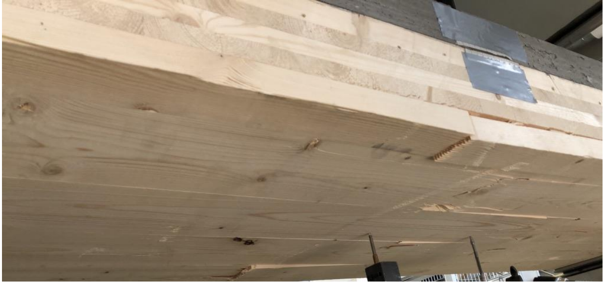
Figure 8-4 Failure in just finger joints and knot separately
