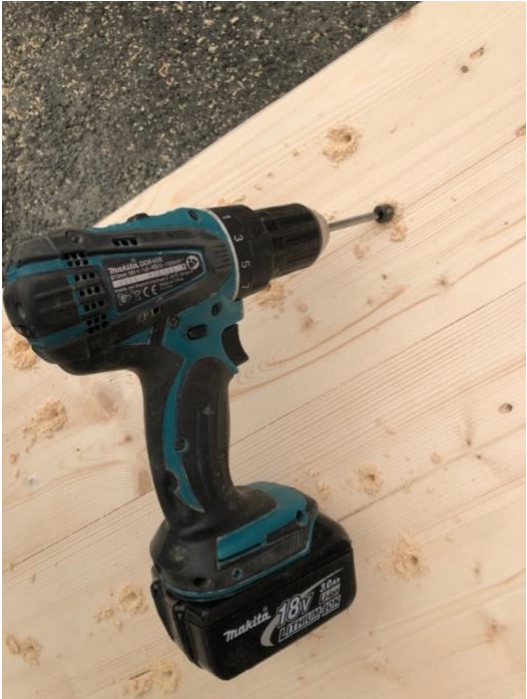
Figure 5-9 Wood drill bit with stop collar in action
