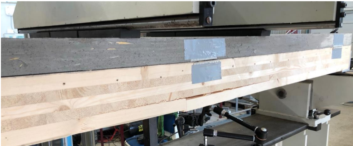
Figure 8-5 Crack in timber at midspan
