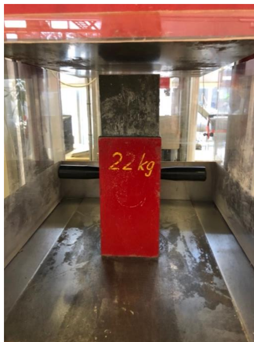
Figure 6-1 Toni-Technik 3000 kN compressive strength test
