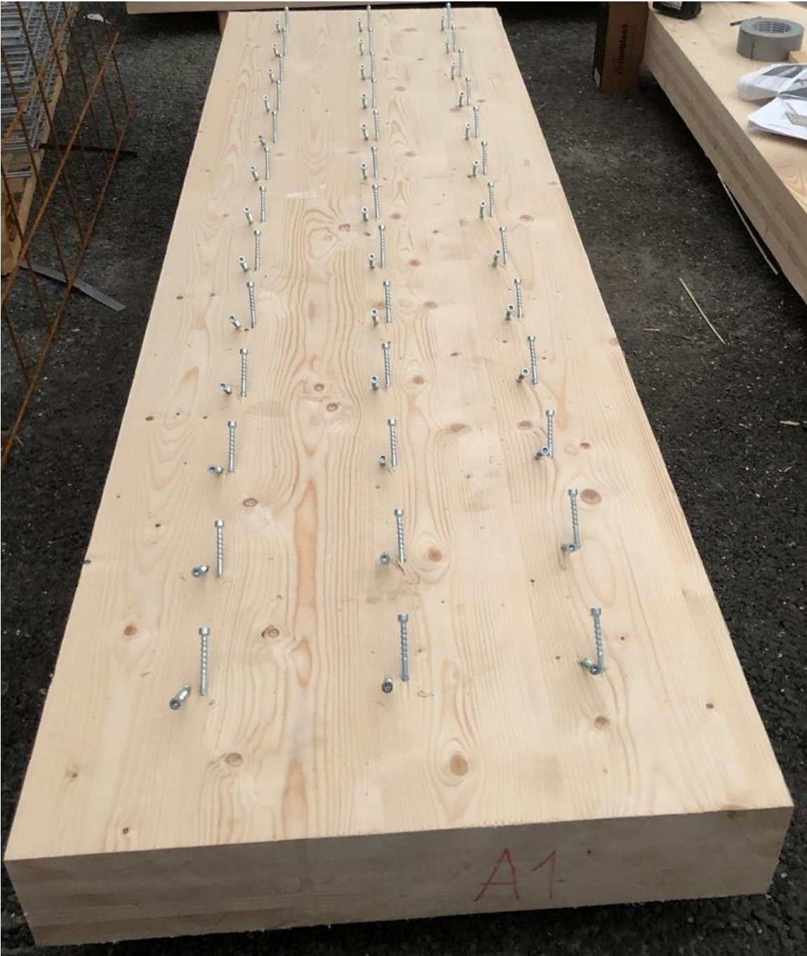
Figure 5-4 A slab with CTC screws - crossed parallel with a 45° angle
