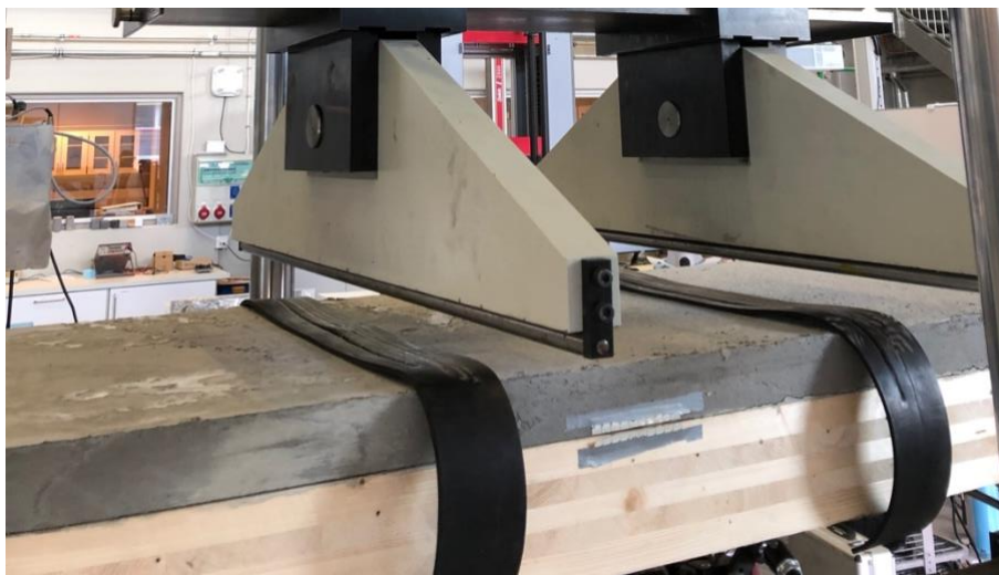
Figure 6-10 Thin rubber pad and placement of ruler
