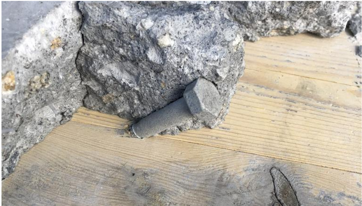
Figure 8-8 KOP screw after four-point bending test
