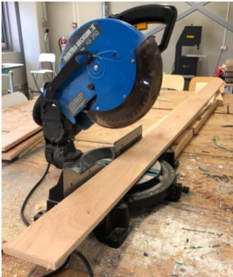
Figure 5-13 Chop saw and the 16 mm plywood used for the formwork
