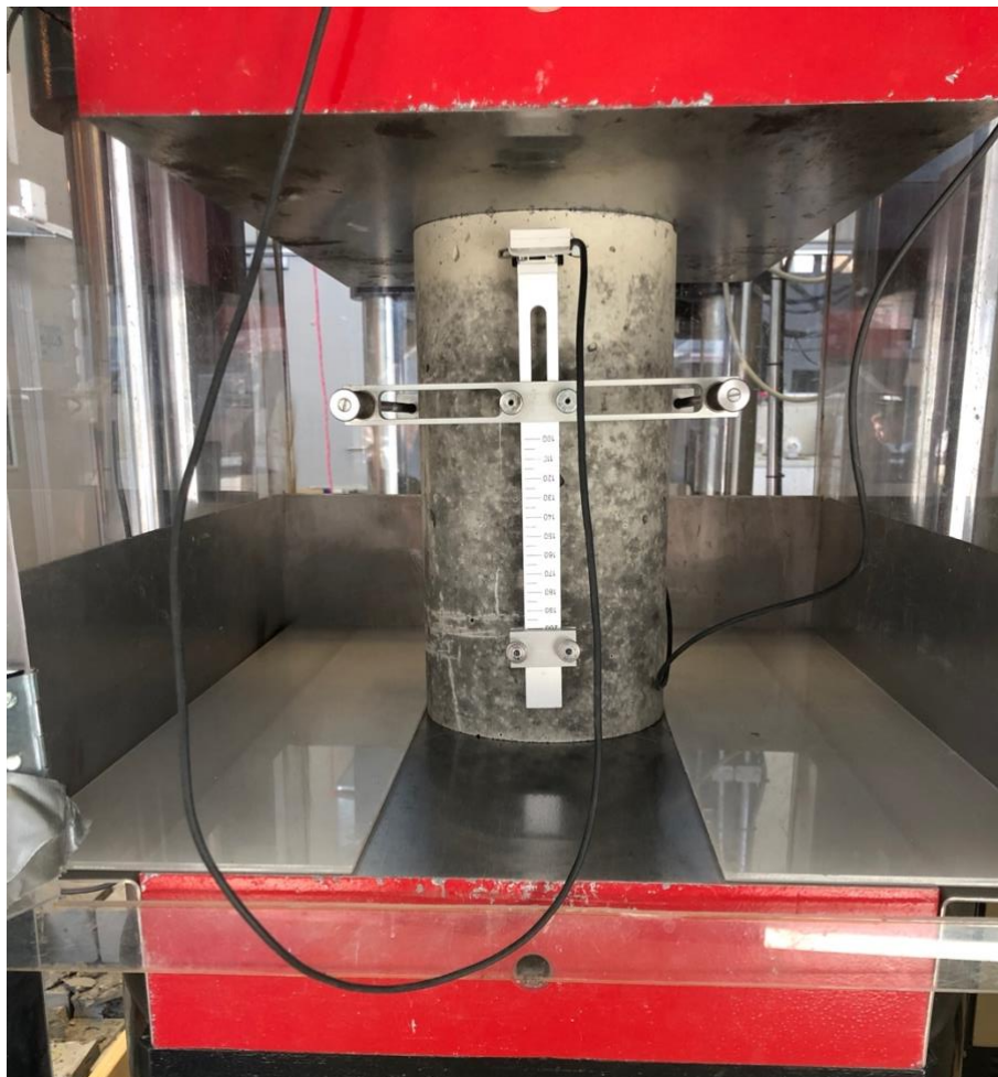
Figure 6-3 Modulus of elasticity testing of a cylinder with deformation measurement device
