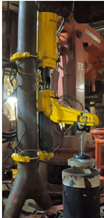
Figure 22 Data While Tripping device mounted the elevator bails of a drilling rig (Vandvik et al., 2021)
