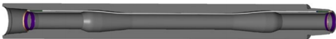
Figure 8 DataCable, running through a joint of pipe, connected to the IntelliCoils (National Oilwell Varco Wellbore Technologies, 2021)
