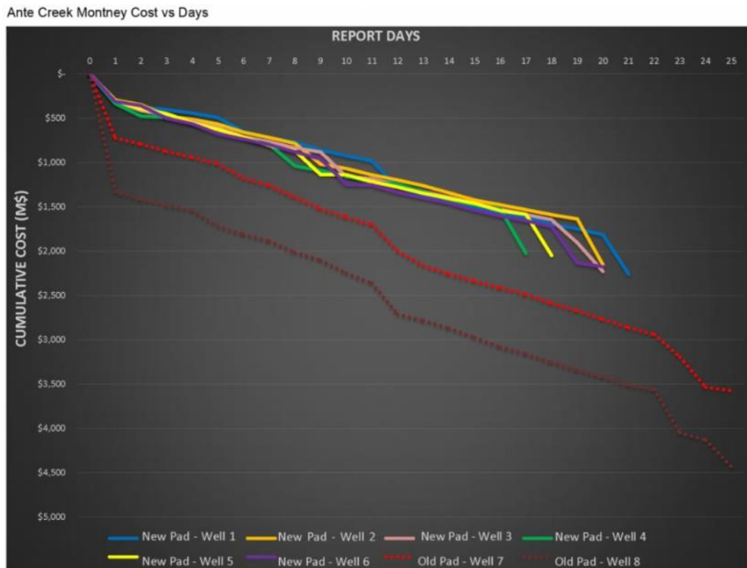
Figure 6.1: The graph shows the cumulative cost vs report days for the 6 well pad compared to the 2 previously wells [53]
