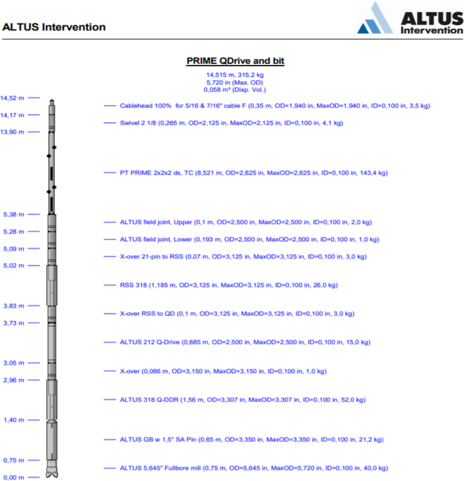
Figure 5.5: Bottom Hole Assembly design [8]
