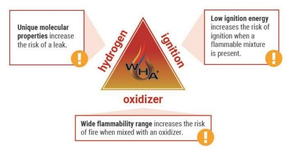
Figure 3. fire or explosion triangle of hydrogen (https://wha-international.com/hydrogen-firerisk-management/)
