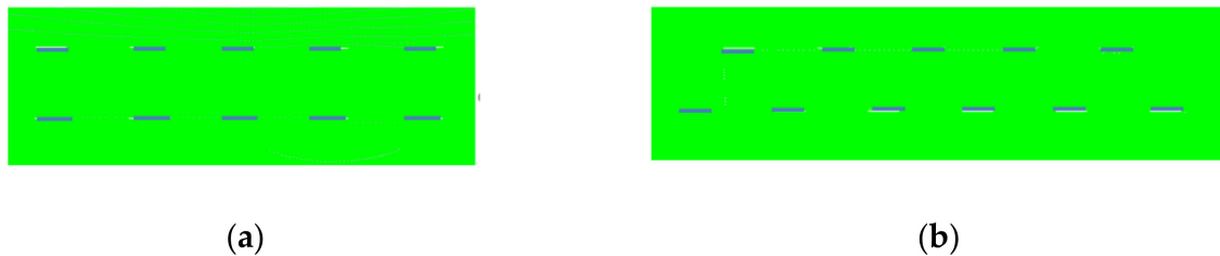
Figure 12. Two different arrangements of wind turbine rows: (a) 5 turbines that are placed directly behind the turbines of the first row; (b) 6 turbines that are facing the gaps between the turbines of the first row.
