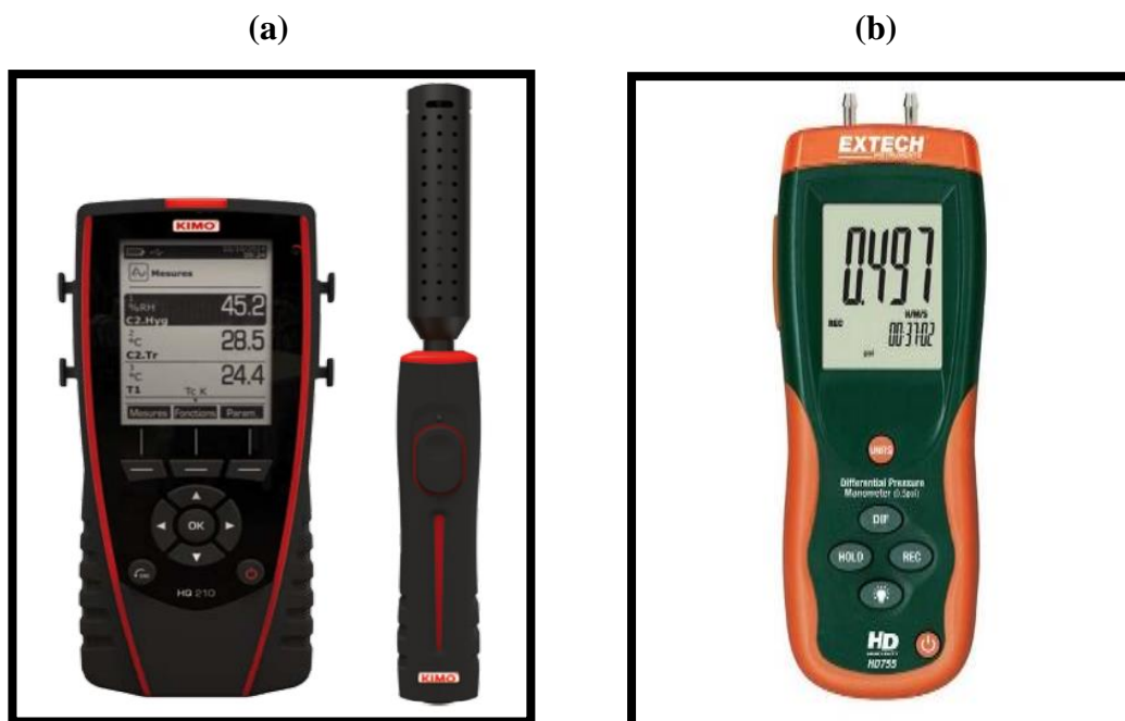
Figure 3.2 (a) KIMO datalogger for measuring the outlet CO 2 concentration from column C-102 (b) Differential pressure manometer used for measuring the pressure drop across C-102
