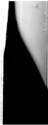
Figure 2.6.1 – Displaying a typical result of Malekmohammadi et al. The black color represents the displacing fluid, while the transparent fluid represents the displaced fluid. An elongated spike on the left side caused by eccentricity is illustrated.
