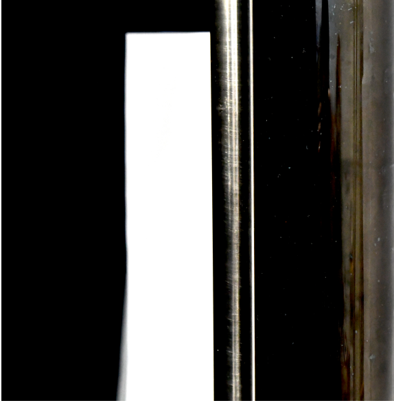
Figure 4.11: Residual water during displacement when Ecc=0.82
