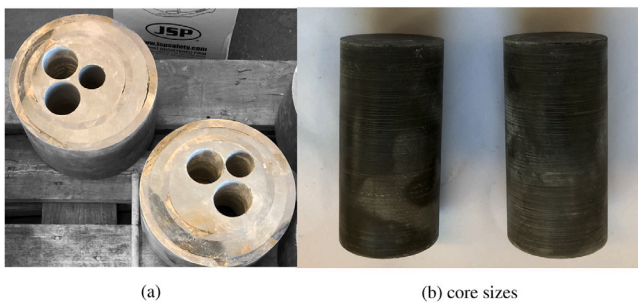
Fig. 3. Specimen preparation process: (a) Coring of cement samples and (b) sizes of cores recovered for testing.
