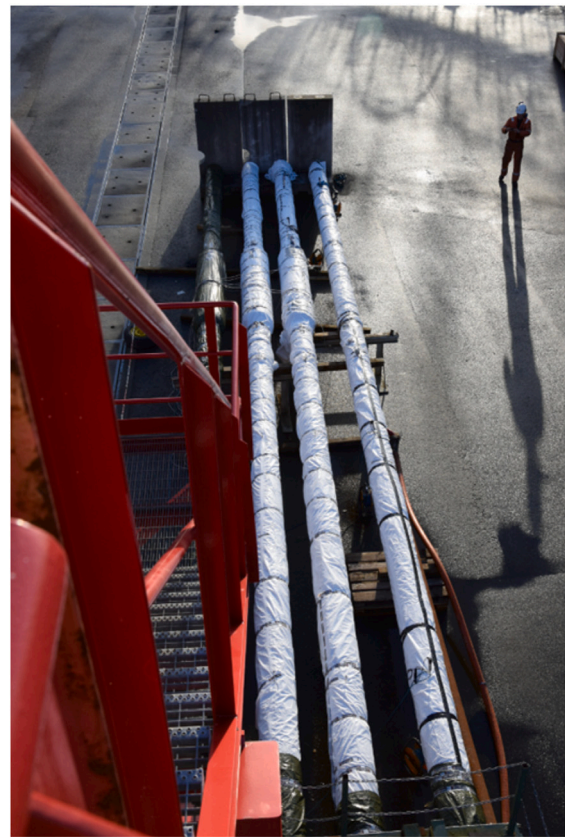
Fig. 1. View of the four test assemblies draped in insulation and plastic covers.
