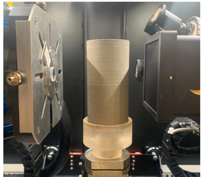
Fig. 7. Oil well cement paste specimen placed between X-ray source and detector.
