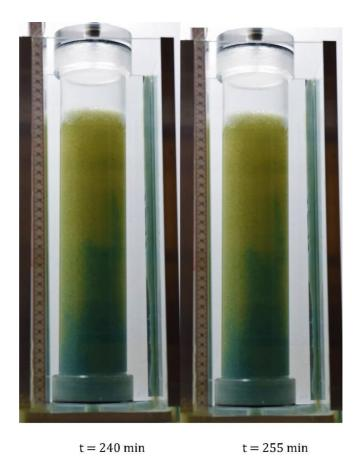
Figure 5.16: Mixing regime from experiment in WSPM of 45% porosity and 23800 mD permeability from t=240 min to t=255 min (Camera 2: Nikon D5300).
