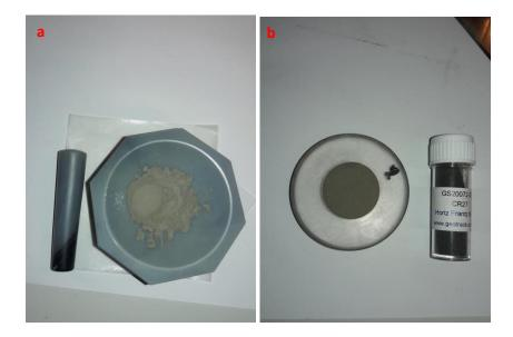
Figure 2.16: An agate-mortar used for milling the sample (a) plastic container used for placing the powder material inside the X-ray diffractometer (b).
