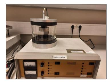
Figure 2.5: Emitech K550 Sputter Coater machine used for coating the mounts before BSE and EDS analysis.
