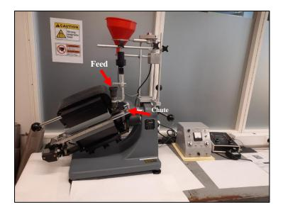
Figure 2.3: Frantz isodynamic separator (Model: LB-1) at UiS Laboratory.
