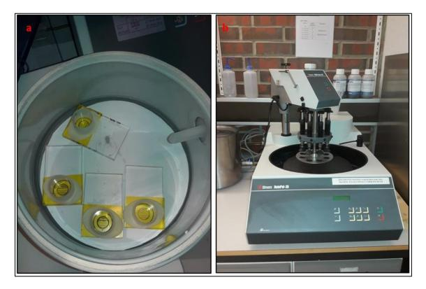
Figure 2.4: Pouring of epoxy on top of grains in a vacuumed chamber (a) the Struers Tegra machine used for polishing sample mounds (b).
