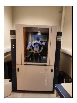
Figure 2.21: The Bruker D8 ADVANCE Eco X-ray diffractometer installed at UiS.
