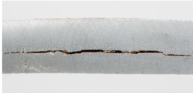
Figure 7. Example of crack propagation due to HISC embrittlement (Uwe Arang, 2014, Creative Commons)
