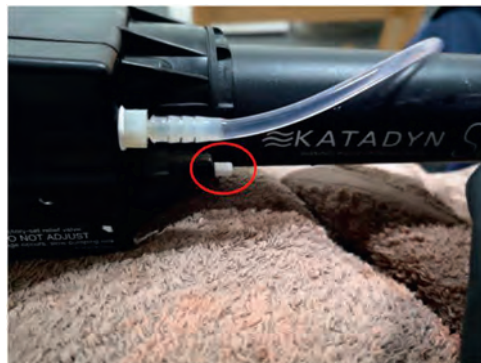
Picture 9. The (white) pressure indicating rod, extending from the (black) indicator housing while pumping. The freshwater outlet hose is seen above. The photo was taken during one of the tests.
