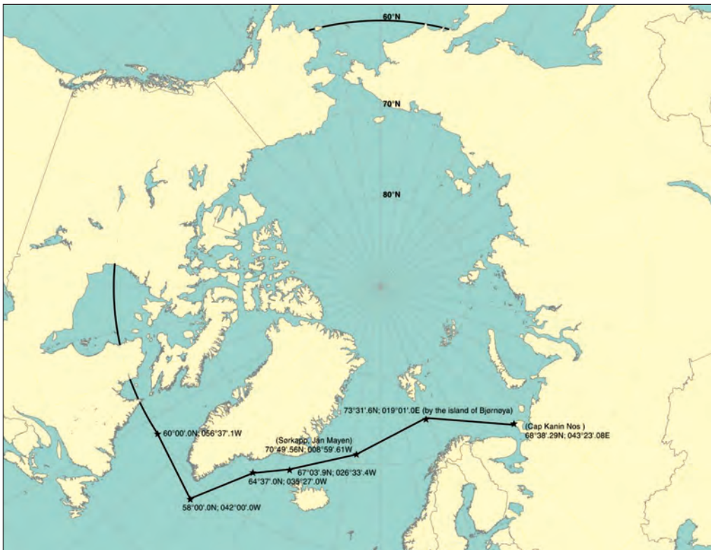
Figure 1. Maximum geographical extent of the Polar Code's area of application in the Arctic. 38
