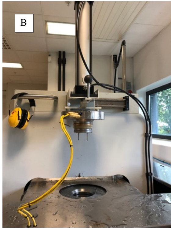
Figure 3.5: A: High pressure machine used to add pressure to merus in order to shuck them. B: Vacuum packaged merus was placed in the chamber with water
