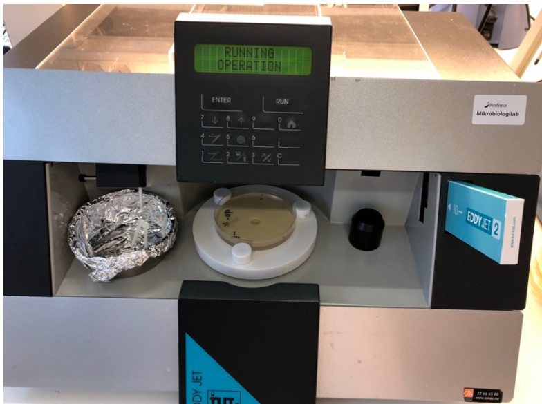
Figure 3.15: Eddy-jet used to spread 10^{-1} and 10^{-3} dilution of the samples on L&H agar.
