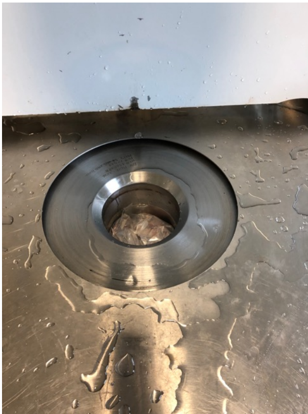
Figure 3.6: Vacuum packaged food placed in the chamber to be high pressure processed by the machine.
