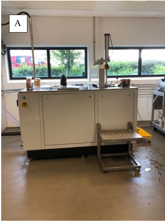
Figure 3.5: A: High pressure machine used to add pressure to merus in order to shuck them. B: Vacuum packaged merus was placed in the chamber with water
