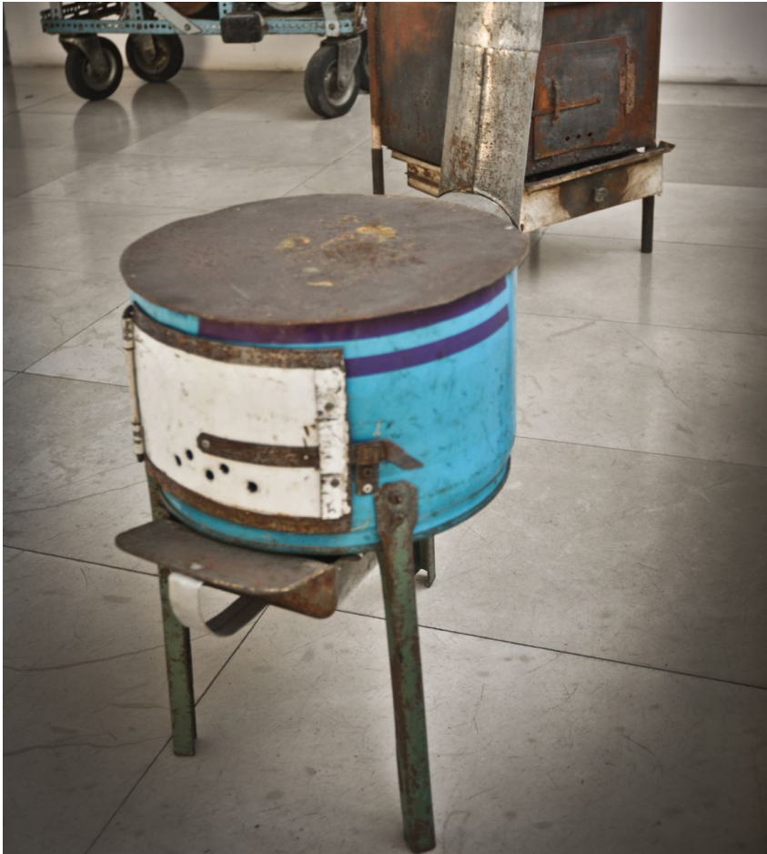
Figure 12 Oven made from a barrel. Historical Museum BiH. Photo by Amar Bidžević, April 2015.
