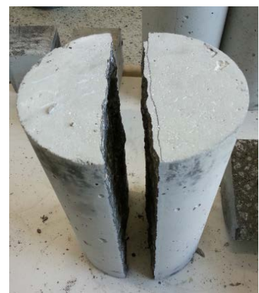
Figur 37: Sylinder splittes i to
