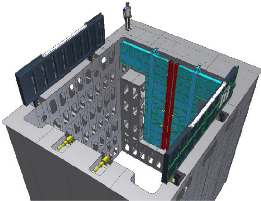
(a) Moonpool hatches in open position. Ready for deployment of modules
