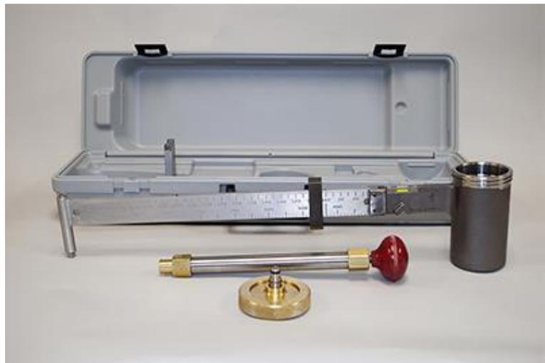
FIGURE 7 MUD BALANCE ([HTTPS://HAMDON.NET/PRODUCTS/TRU-WATE-MUD-BALANCE-MODEL-141](https://hamdon.net/products/tru-wate-mud-balance-model-141))
