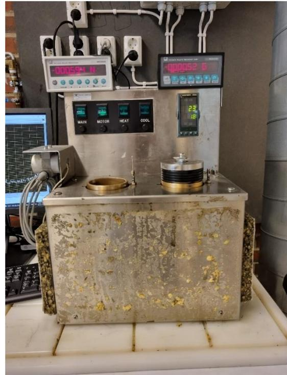
FIGURE 4 ATMOSPHERIC CONSISTOMETER PRIVATE PHOTO
