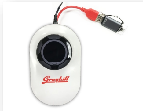
Connect USB to Red Cable, Power on
