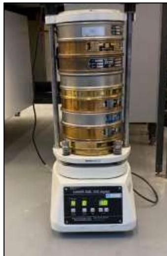
Figure 3.5: Haver EML 200 Sieving equipment.
